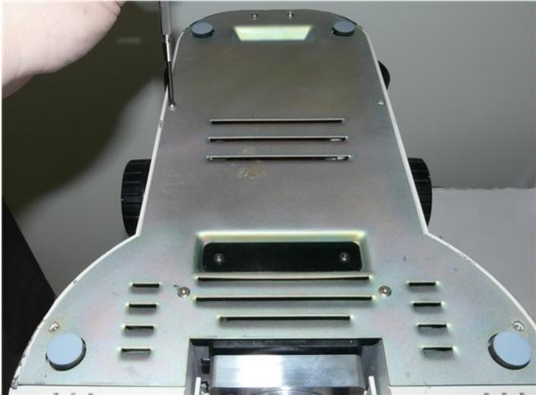
(4) Install the rest of the screws. The two just under the black filter holder need a 1.5mm hex key. The other 6 need a phillips screwdriver.
