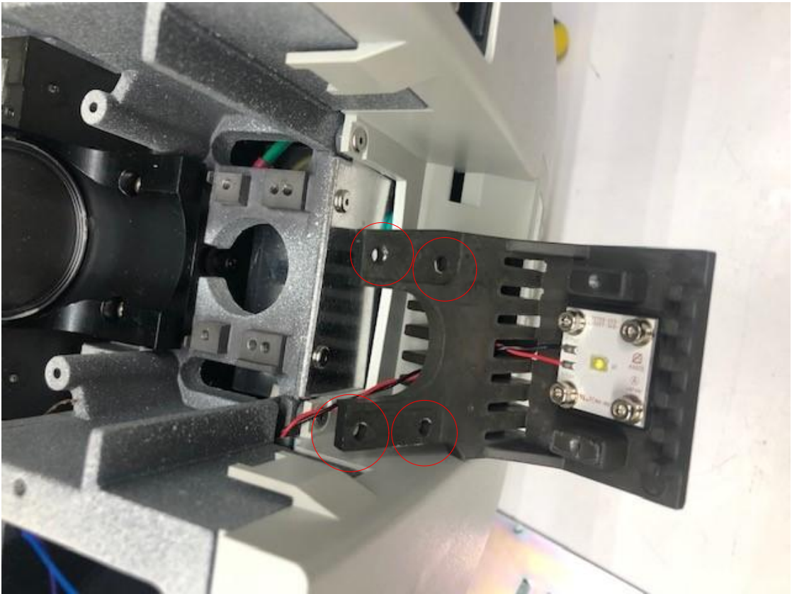
(3) Remove the filter (red circle) so it does not fall out if you turn the scope over.
