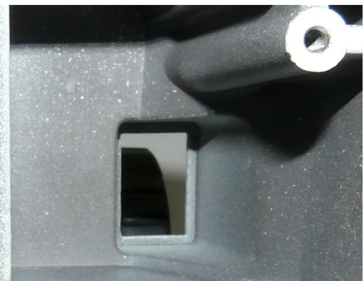
(4) Remove the power switch. Use tweezers or a small screw driver to compress the plastic retainers holding it in place while pushing it out.
