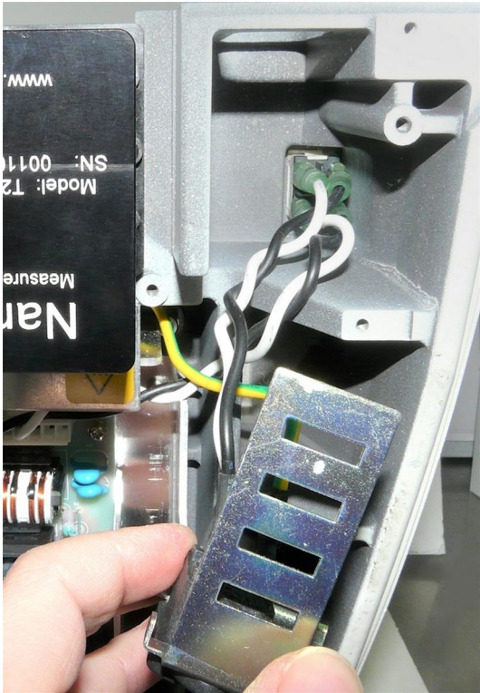
(1) Unscrew the obsolete AC power bracket and pull it away from the microscope.
