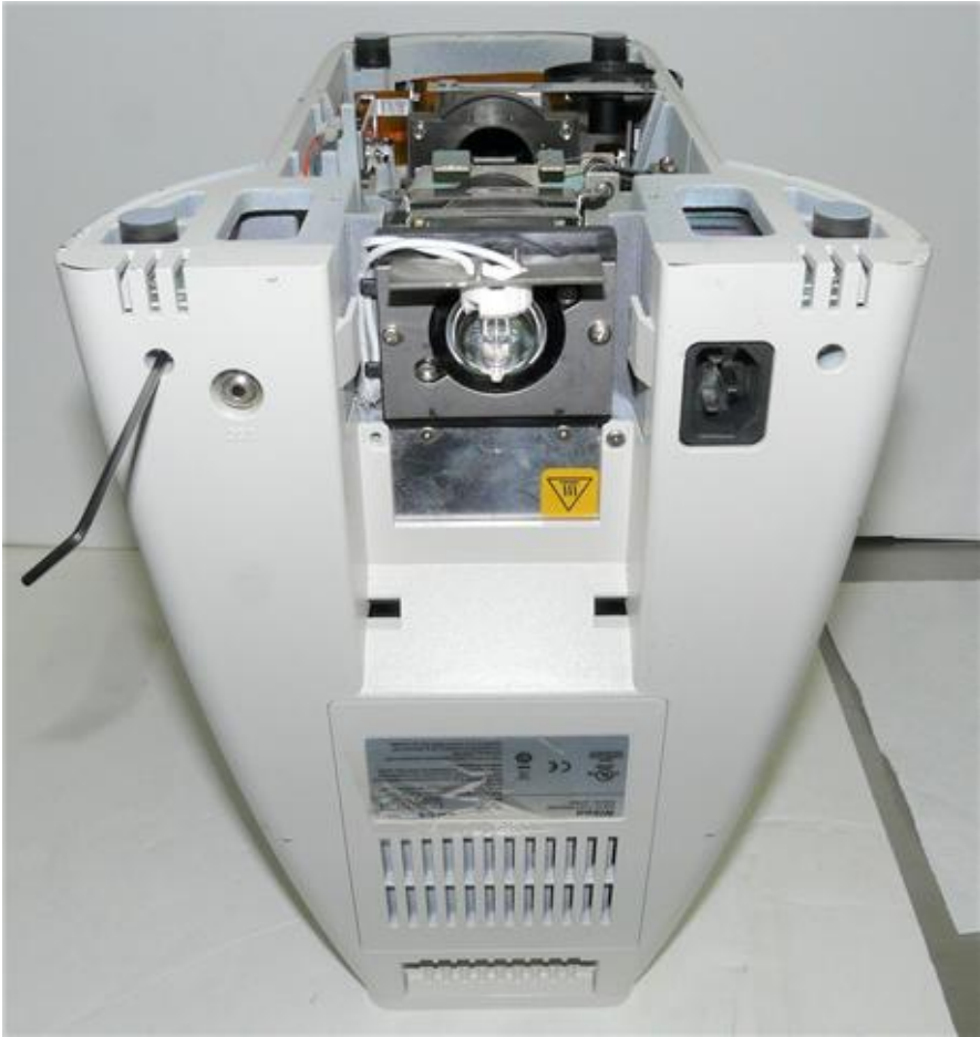
(4) Remove the back cover (6 screws).
