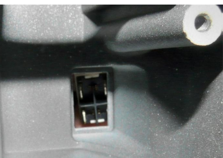
(1) Unscrew the obsolete AC power bracket and pull it away from the microscope.
