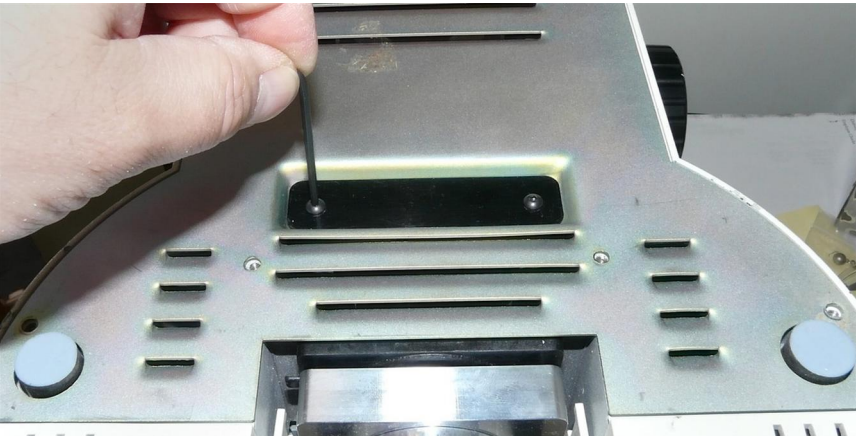
(3) Replace the bottom cover and tighten the black screws for holding the filter. (use a 2mm hex key)
