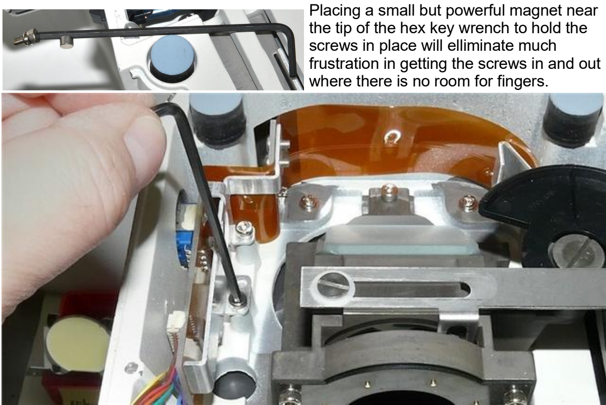
(1) Original illuminator removed. (2) Unplug the intensity cable and pull it out of the microscope as shown. (3) Loosen the set screw on the pot knob. Remove and save it.
