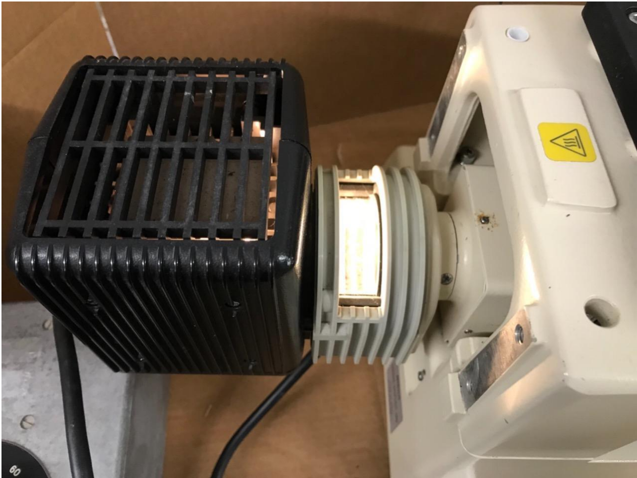
(2) This replaces the Nikon Epiphot 200 100W illuminator. If the original lamp house looks like this photo, this illuminator system is the right one for you.
