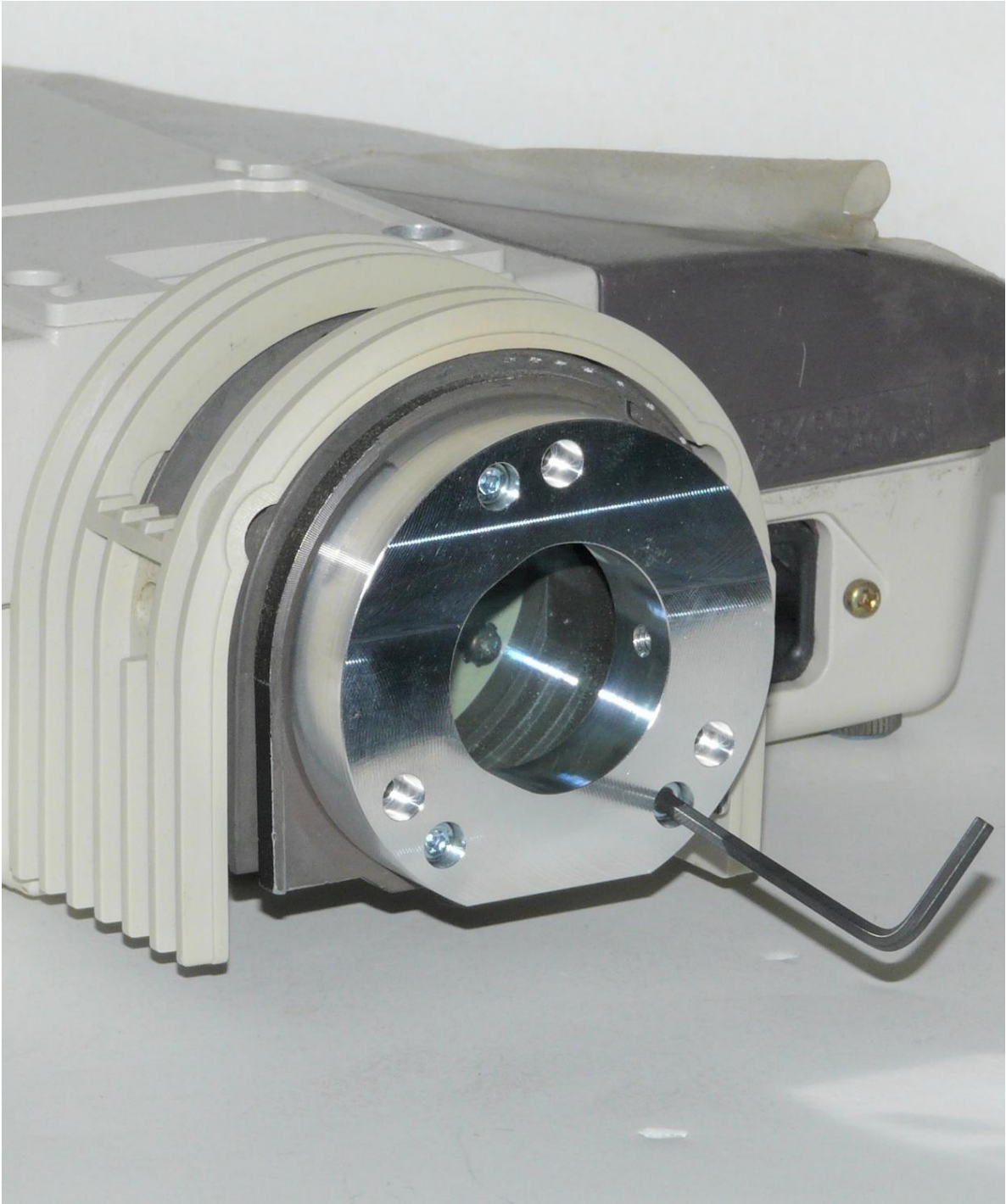
(2) Attach the adapter ring using the three 12mm long M3 screws, using the 2.5mm hex key.
