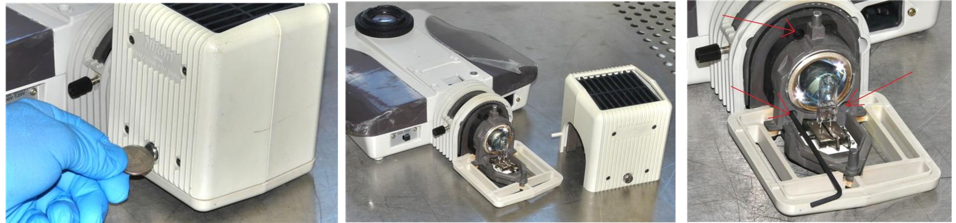
(1) Loosen the screw holding the lamp cover. (2) Lift the cover off the lamp housing. (3) Remove the 3 screws holding the lamp housing to the microscope with the 2.5mm hex key provided.
