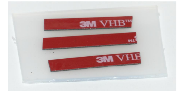
Tape to secure wires.
