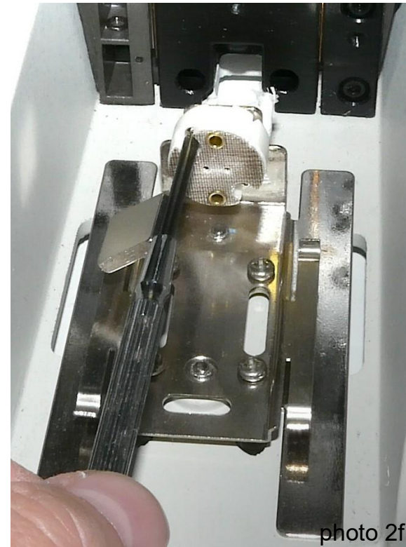
(1) Unscrew and remove the heat shield from the collector lens/lamp housing assembly. (it interferes with the power cable on the new assembly)
