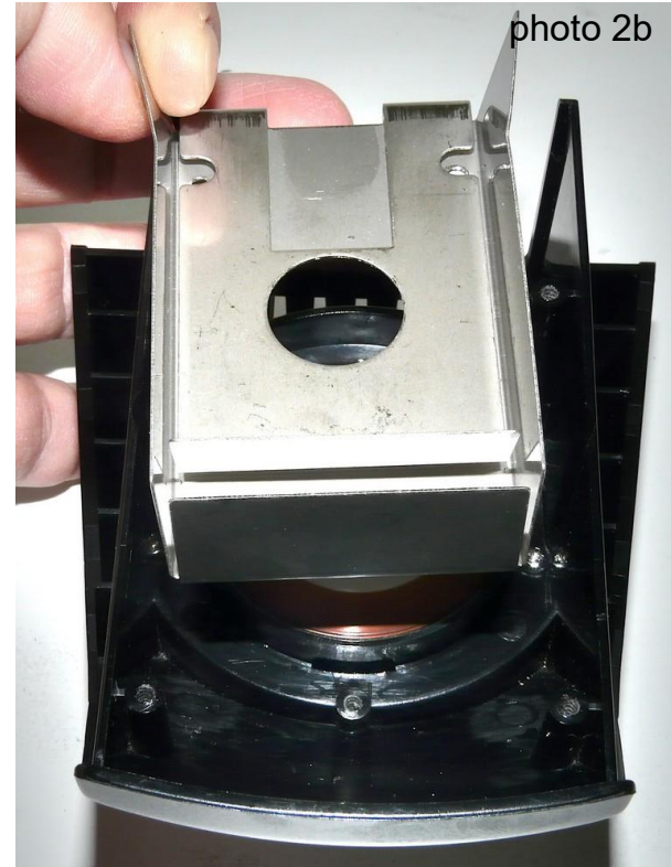
(1) Unscrew and remove the heat shield from the collector lens/lamp housing assembly. (it interferes with the power cable on the new assembly)
