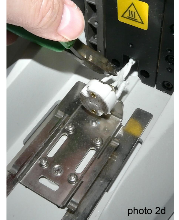
(3) Cut the wires from the OEM lamp socket.
