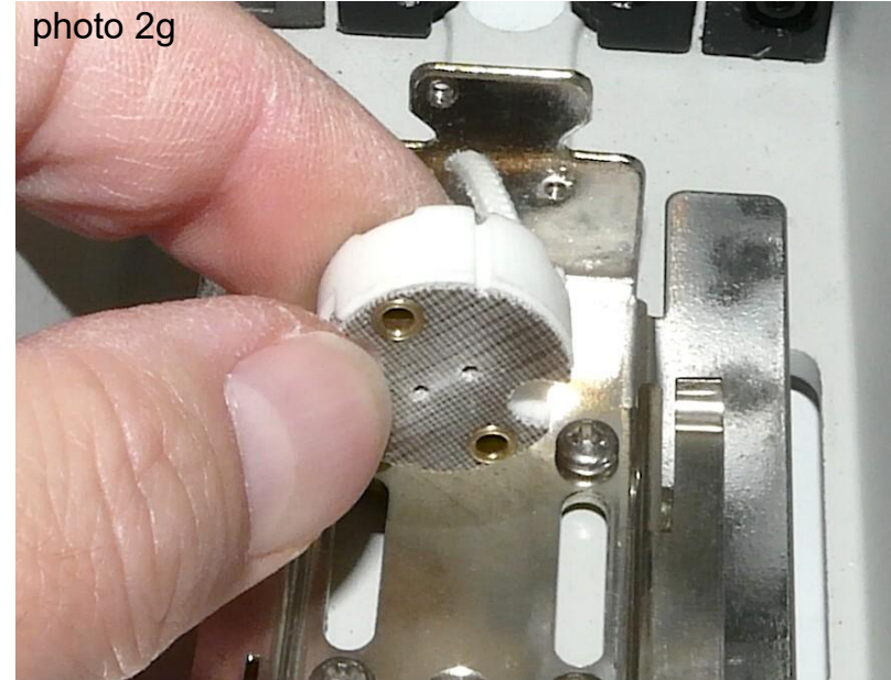
(5) Remove the screws holding the socket with a phillips screwdriver (photo at left). Then remove the socket (photo above).
