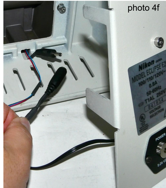
(5) Install the new DC power receptacle using the M3 button head screws provided.
