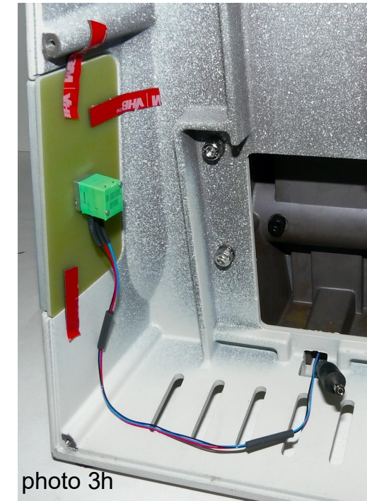
(6) Install the new adjustment pot plate assembly. (2 photos at left)
