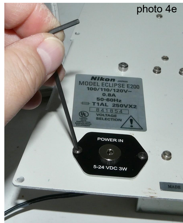
(5) Install the new DC power receptacle using the M3 button head screws provided.
