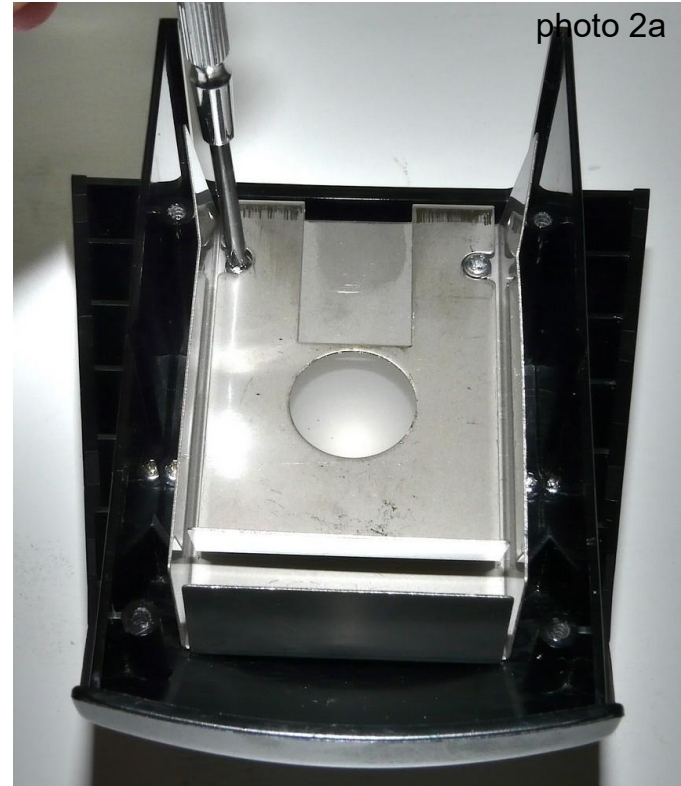
(1) Unscrew and remove the heat shield from the collector lens/lamp housing assembly. (it interferes with the power cable on the new assembly)
