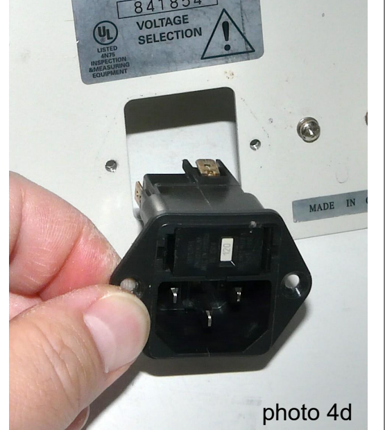
(4) Remove the original AC power receptacle from the back cover.
