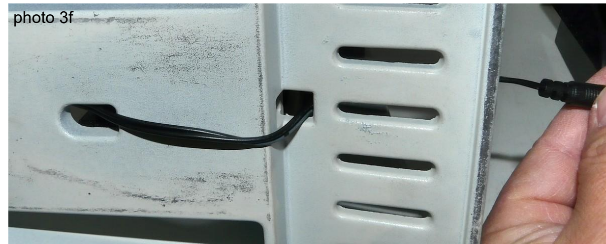
(5) Route the cable as shown in photo 3f.
