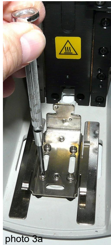
(1) Remove the four screws holding the metal railing. Leave the railing in place.
