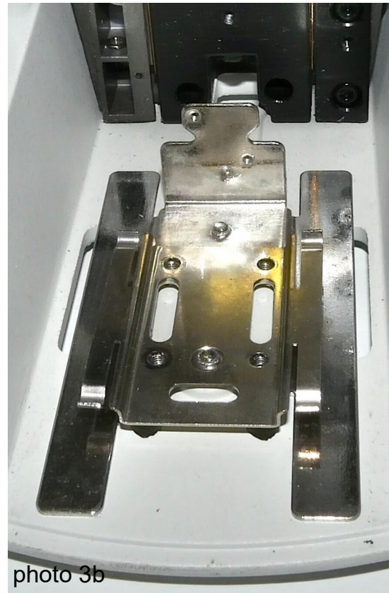
(1) Remove the four screws holding the metal railing. Leave the railing in place.
