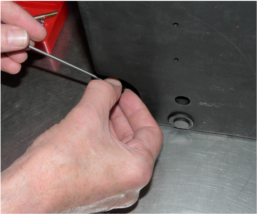
(4) Install the knob on the new pot using the 2.5mm hex key provided.
