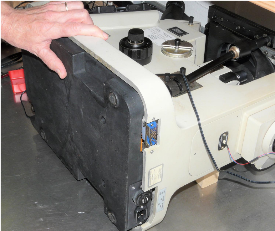
(5) Replace the bottom cover.
