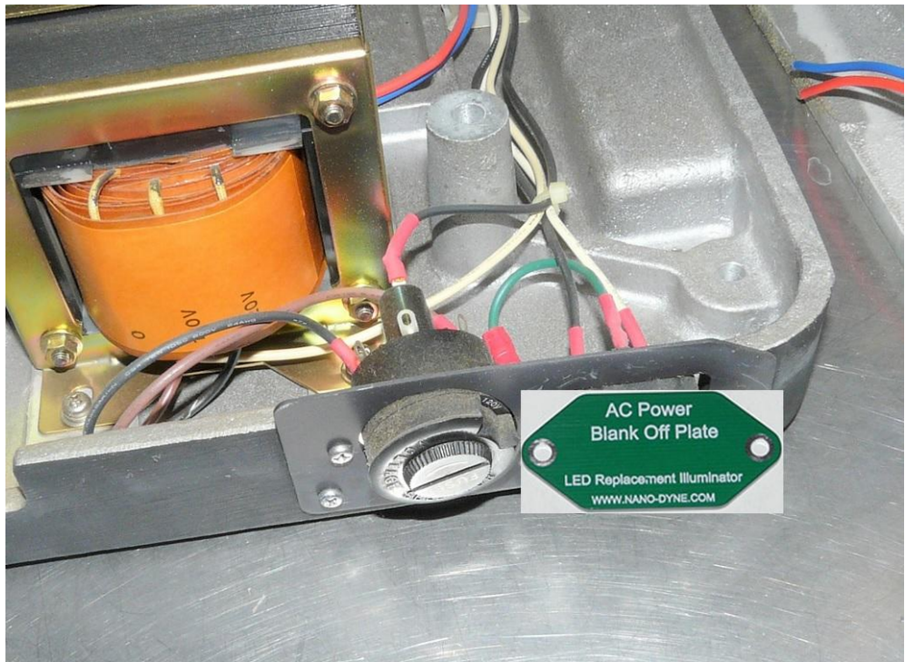
(1) Connect the power supply cable to the wall mount and plug in to the Nanodyne illuminator.
