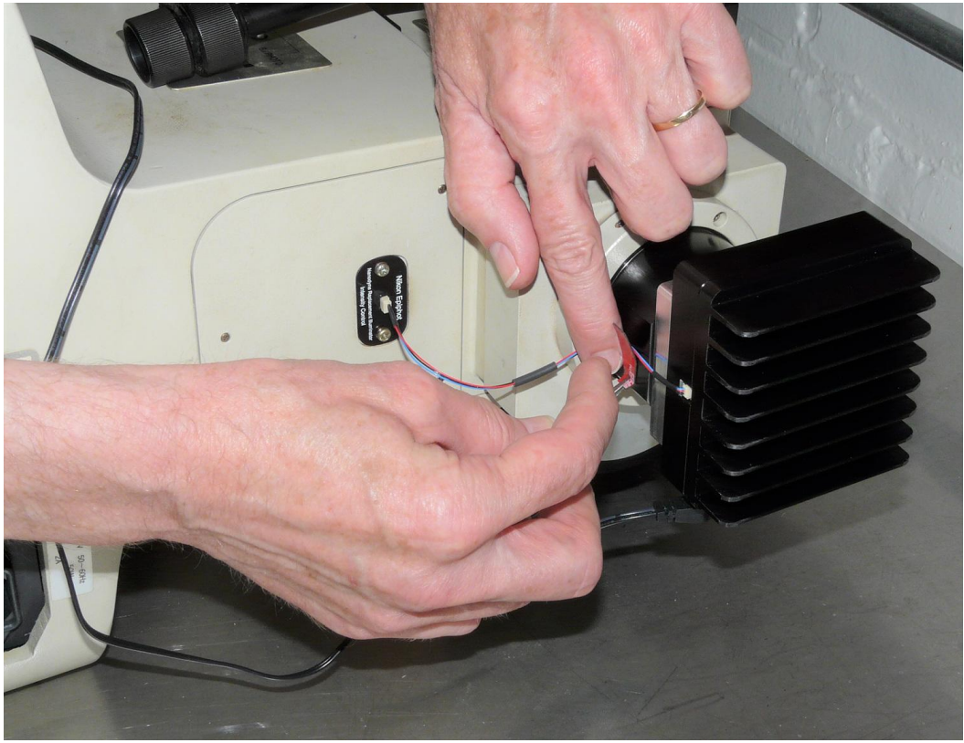
(2) Secure the pot cable with the 3M VHB tape provided (red, in above photo).
