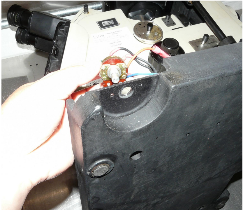
(3) Remove the old potentiometer.
