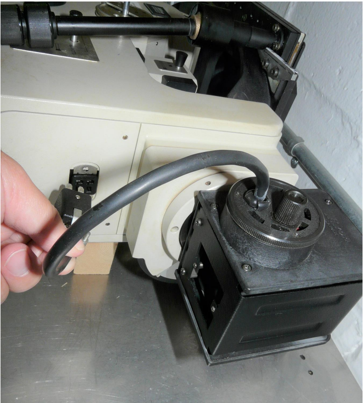
(1) Be sure the AC power is unplugged. Disconnect the original lamp power cable.
