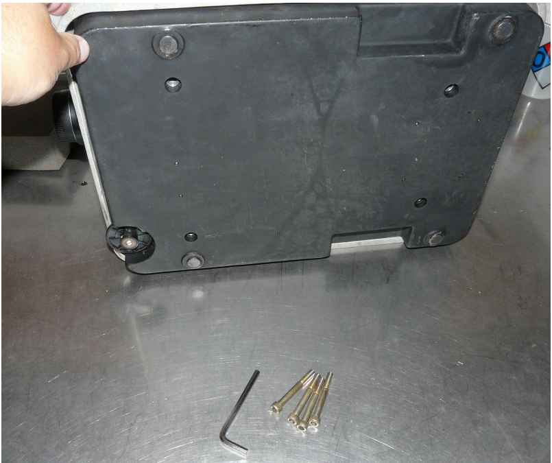
(3) Remove the 4 screws holding bottom cover using 5mm hex key provided and open the bottom cover. Keep the screws for later.
