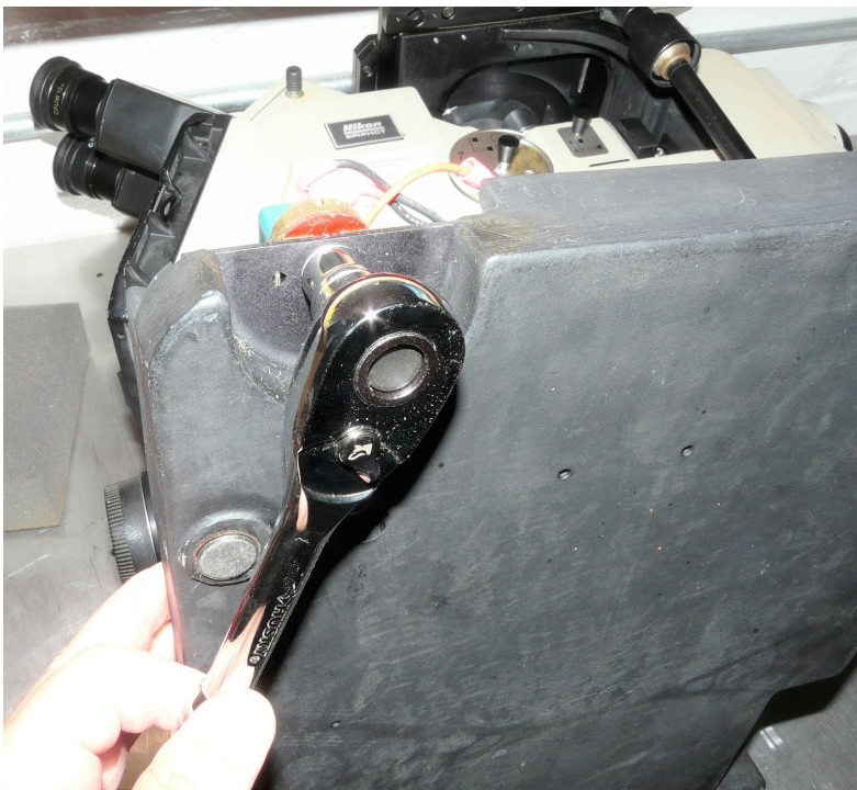
(1) Unscrew the nut holding the old pot, using a hex socket.
