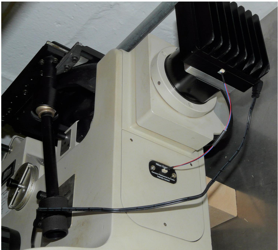
(1) Connect the power supply cable to the wall mount and plug in to the Nanodyne illuminator.
