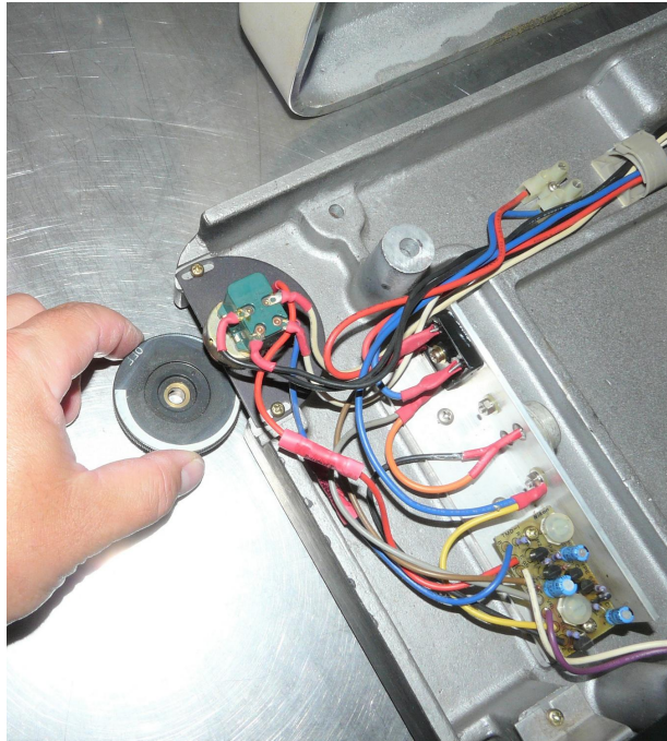
(6) Remove the knob using the 2.5mm hex key provided. Save the knob for the new pot.
