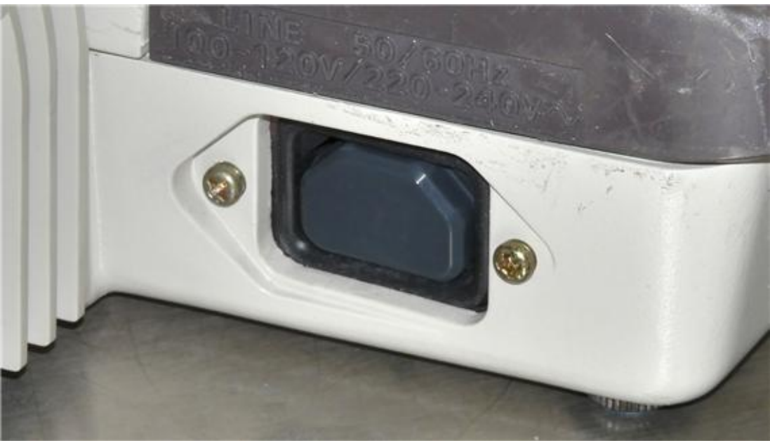
(4) Silicone rubber blocking plug installed in AC power receptacle.
