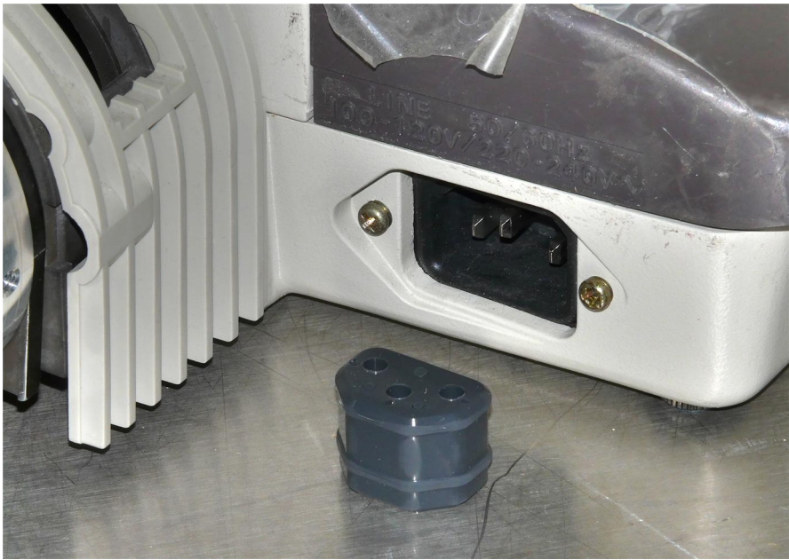
(3) Silicone rubber plug provided to block the AC power receptacle if no longer needed.
