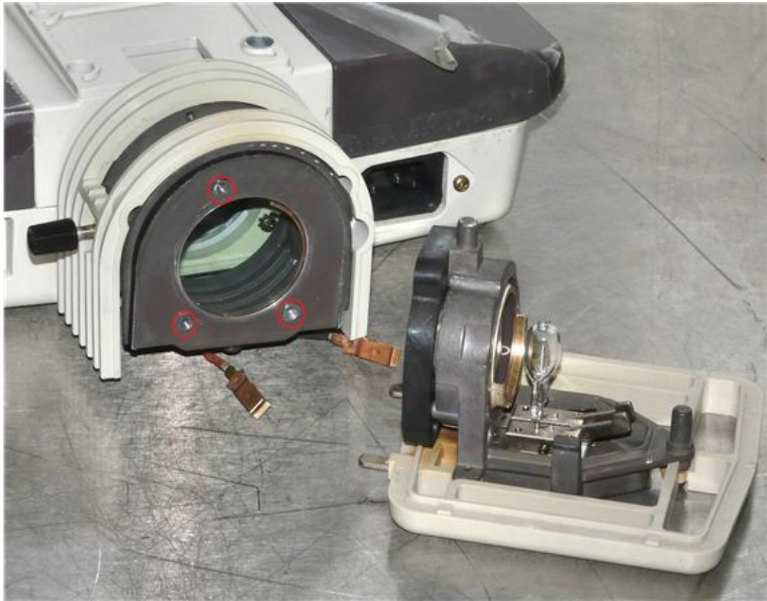
(1) Loosen the screw holding the lamp cover. (2) Lift the cover off the lamp housing. (3) Remove the 3 screws holding the lamp housing to the microscope with the 2.5mm hex key provided.
