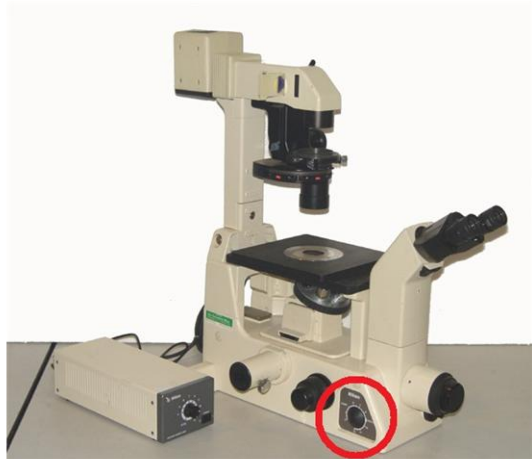
(2) Remove the knob, then remove the old pot.
