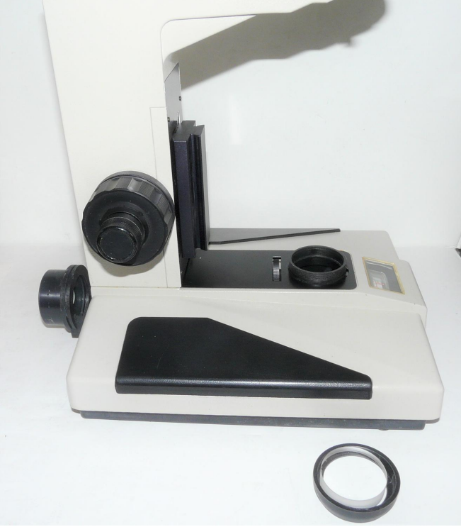
(2) Remove the 4 screws holding bottom cover using 4mm hex key provided. Keep the screws for later.
