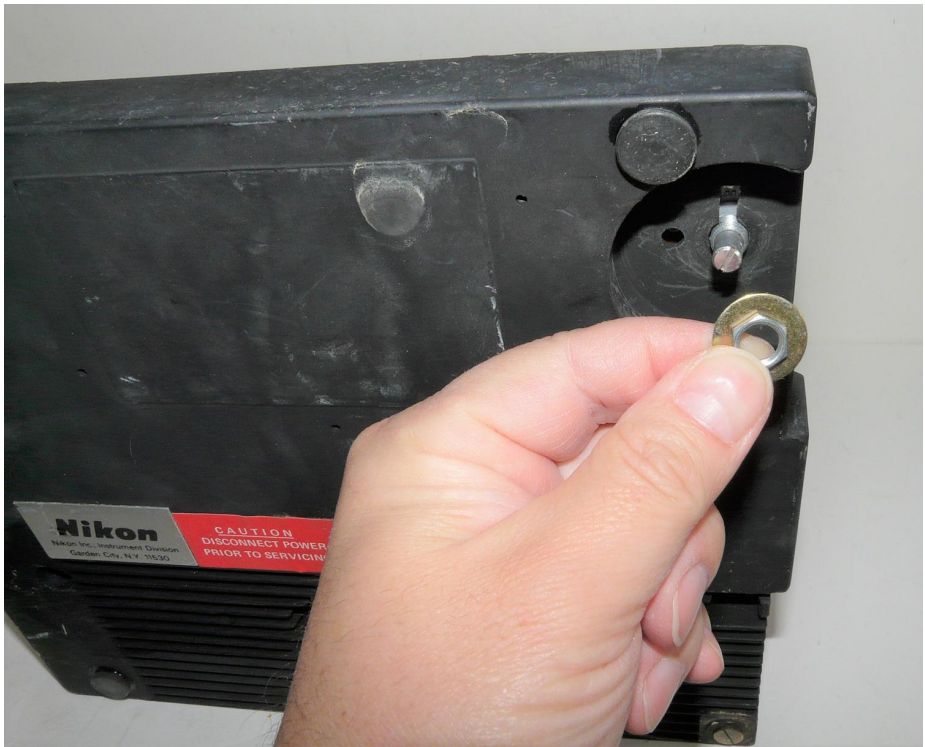
(6) Remove the washer and nut.
