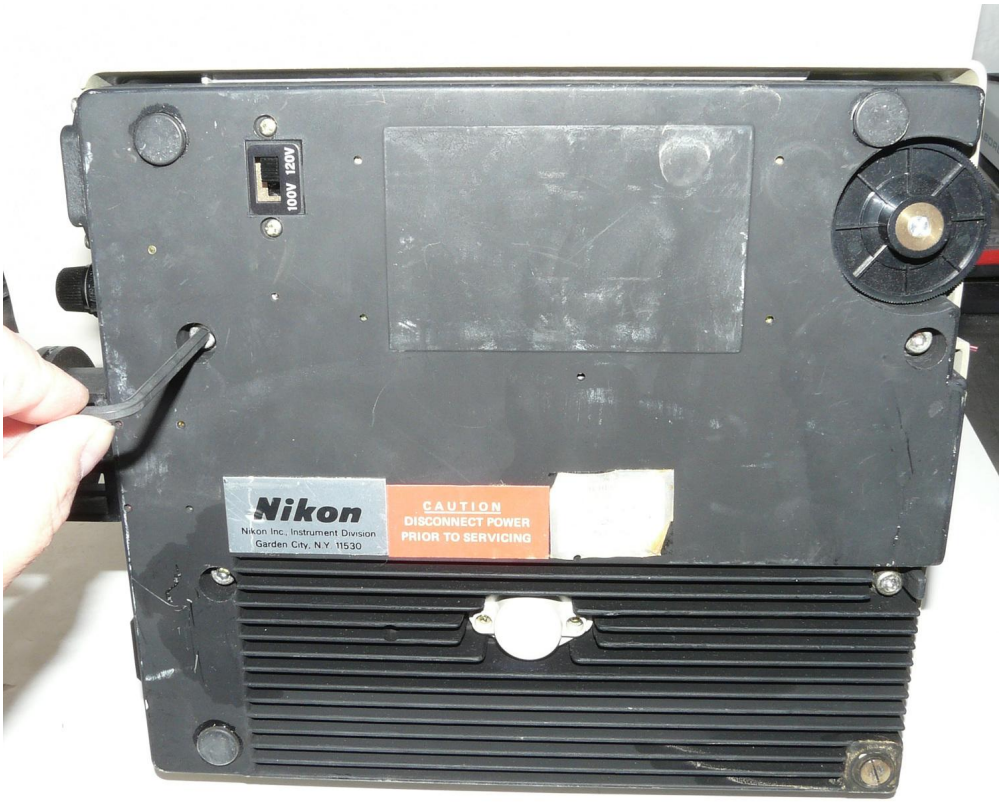
(2) Remove the 4 screws holding bottom cover using 4mm hex key provided. Keep the screws for later.
