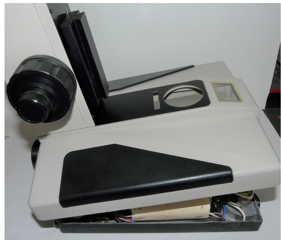
(1) Take the microscope frame off.
