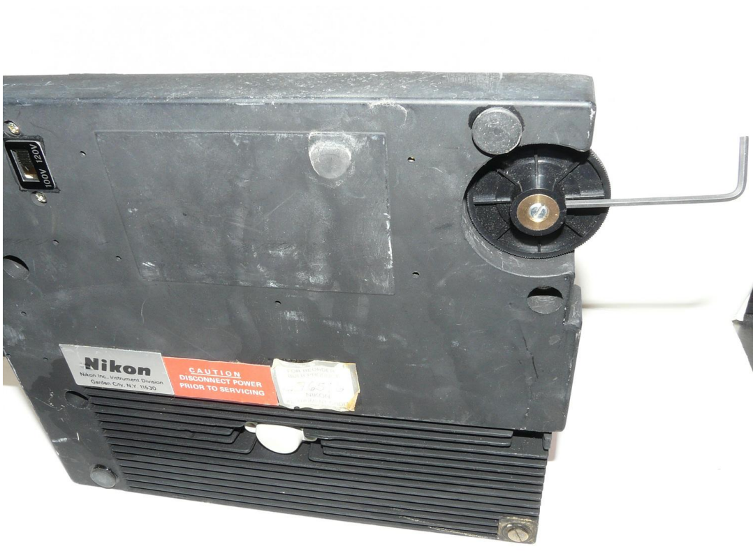
(3) Loosen the set screw on the pot knob using 2.5mm hex key provided.
