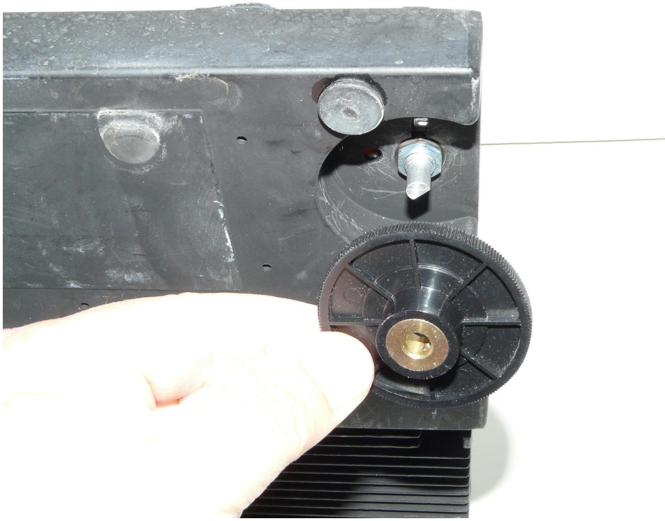
(5) Reinstall the knob on the new pot.
