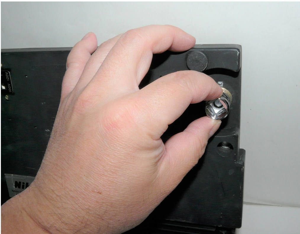
(5) Unscrew the nut using the 10mm hex socket.
