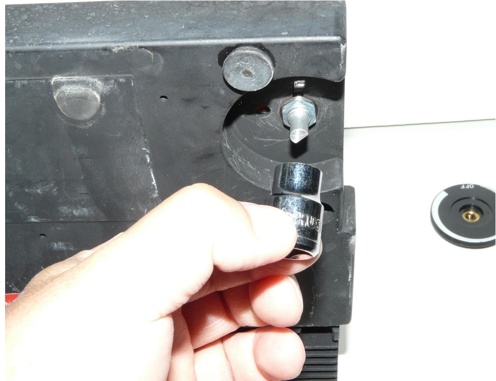
(4) Secure the new pot in place with the nut and washer provided. You should be able to turn the nut by hand. If it is too difficult, a hex socket or other tools may be required.
