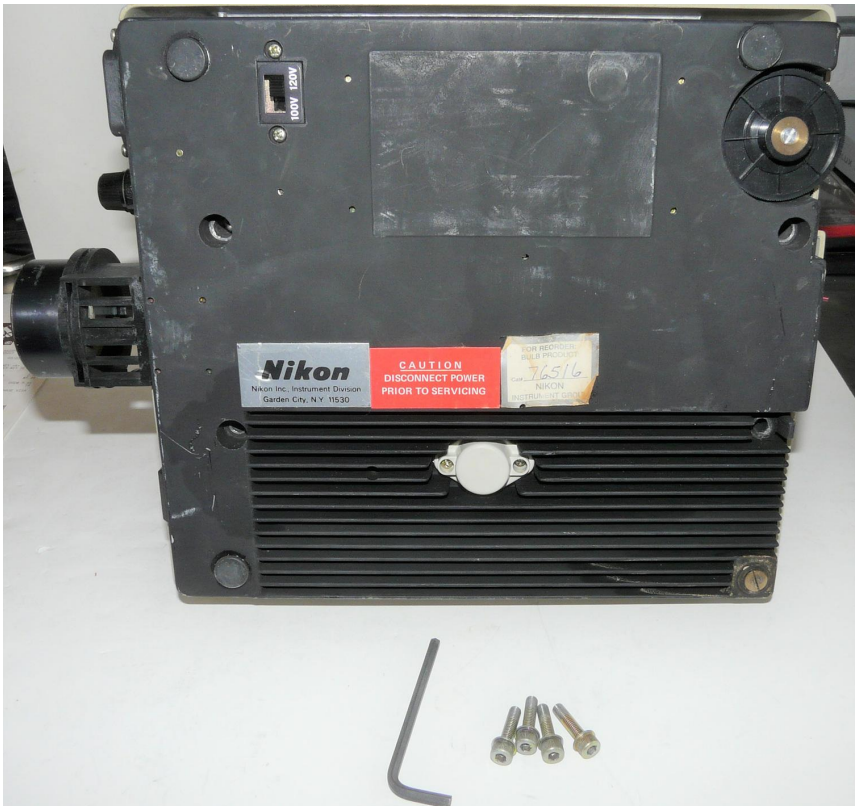
(2) Remove the 4 screws holding bottom cover using 4mm hex key provided. Keep the screws for later.
