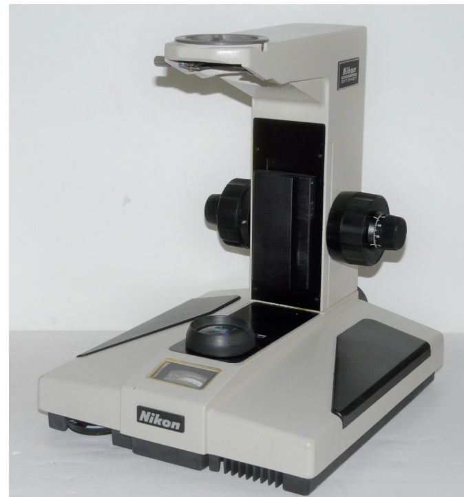
(6) Replace the microscope frame. Tighten the 4 screws saved. Connect the power supply cable to the wall mount and plug in to the Nanodyne illuminator. The microscope is now ready to operate.
