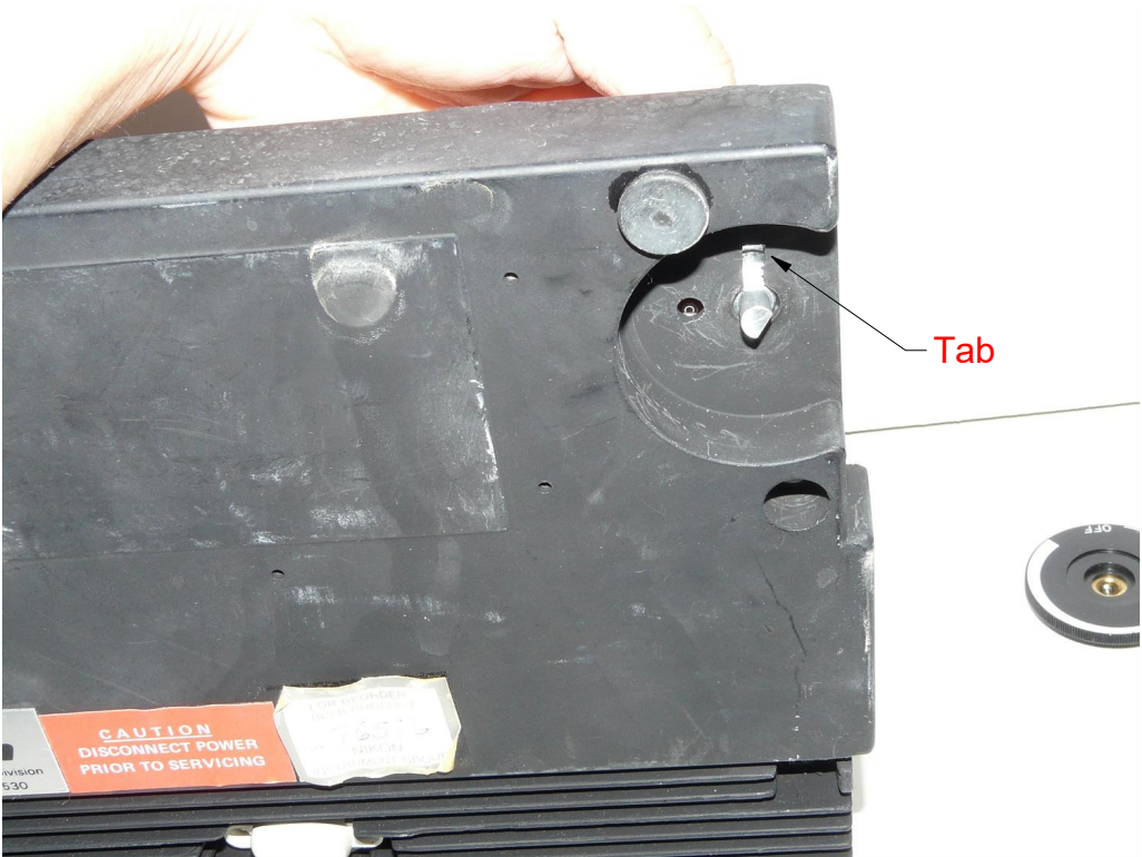
(3) Install the new potentiometer. Align the tab into the hole.
