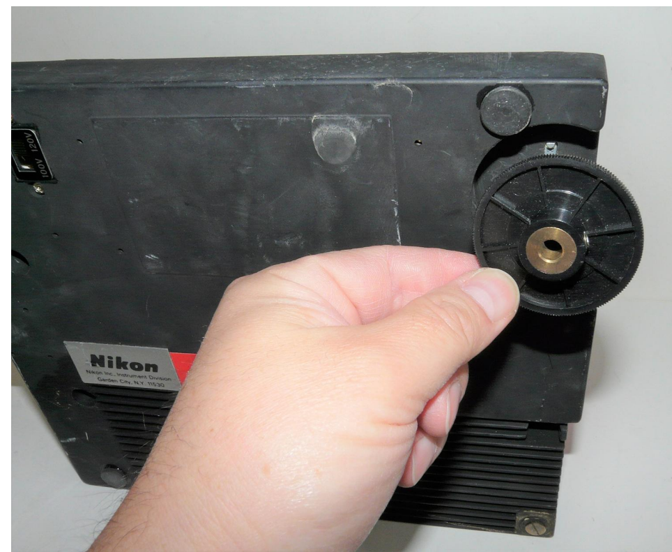
(4) Remove the knob. Save the knob for the new pot.
