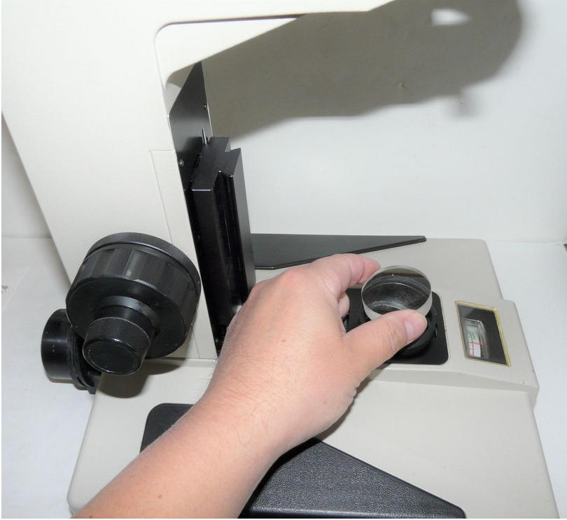
(3) Unscrew and remove the lens assembly by hand. Keep the parts for later.
