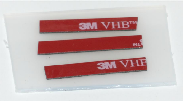
3M VHB tape to secure pot cable
