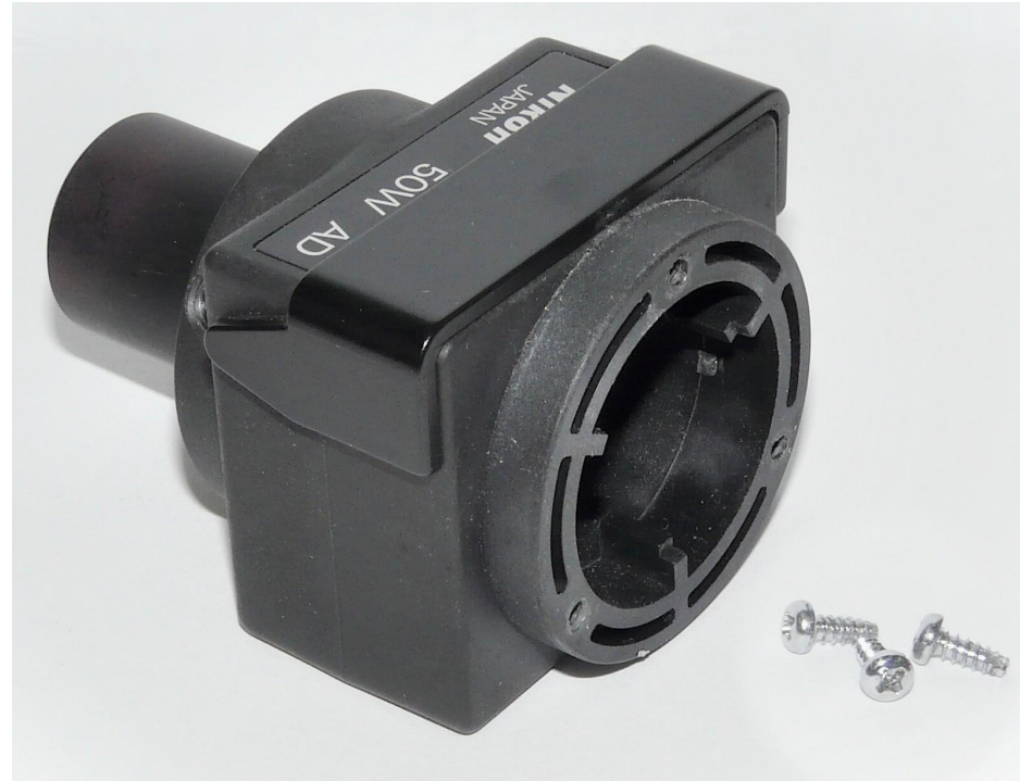
(1) Remove the lamp house assembly from the collector lens/filter holder assembly of the original illuminator as shown above.
