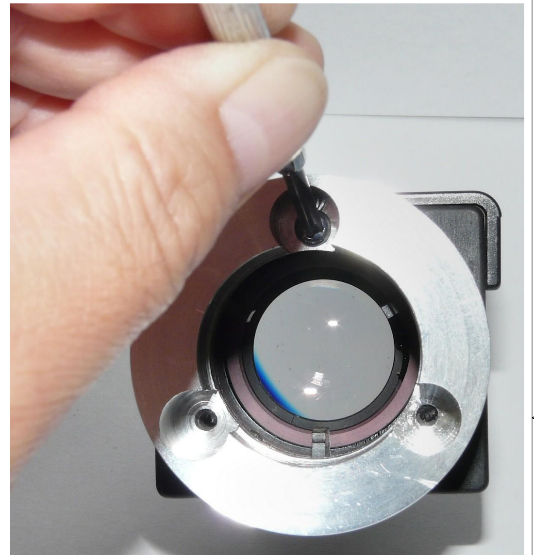
(3) Attach the Nanodyne mounting adapter to the collector lens/filter holder assembly from the microscope. Use the screws from the original illuminator.
