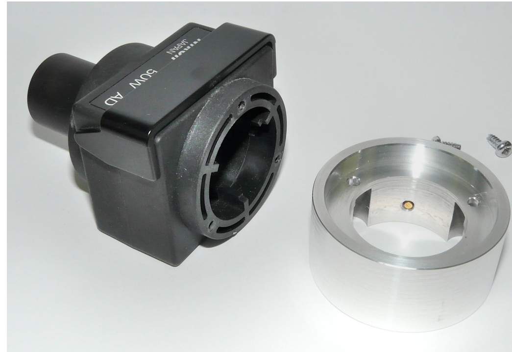
(2) The Nanodyne mounting adapter will be attached to the collector lens/filter holder assembly from the microscope.
