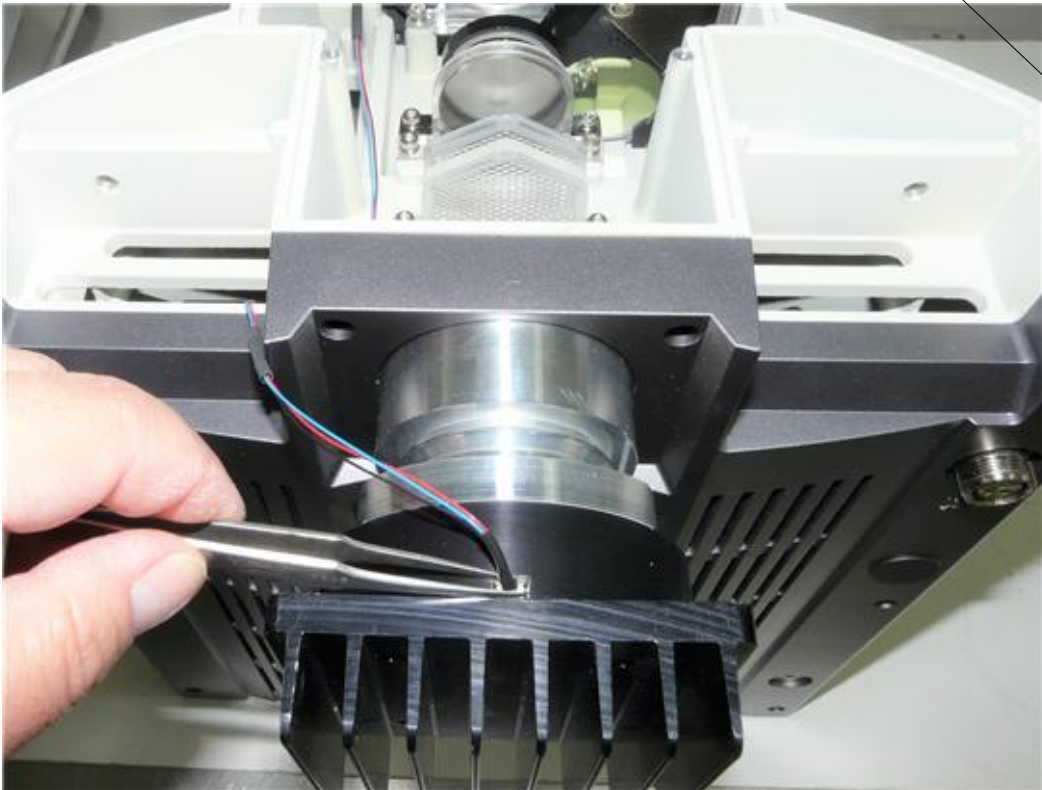
(4) Connect the pot cable to the illuminator.
