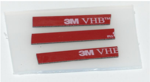
3M VHB tape to secure pot cable
