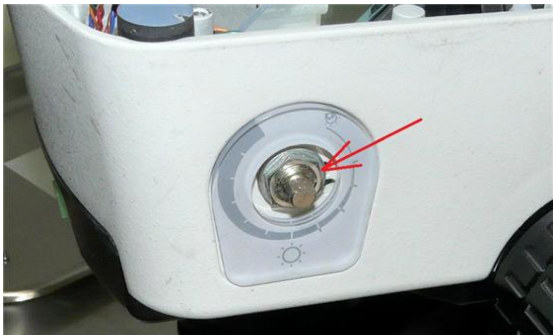
(6) Remove the nut holding the old pot, using a 12mm socket.
