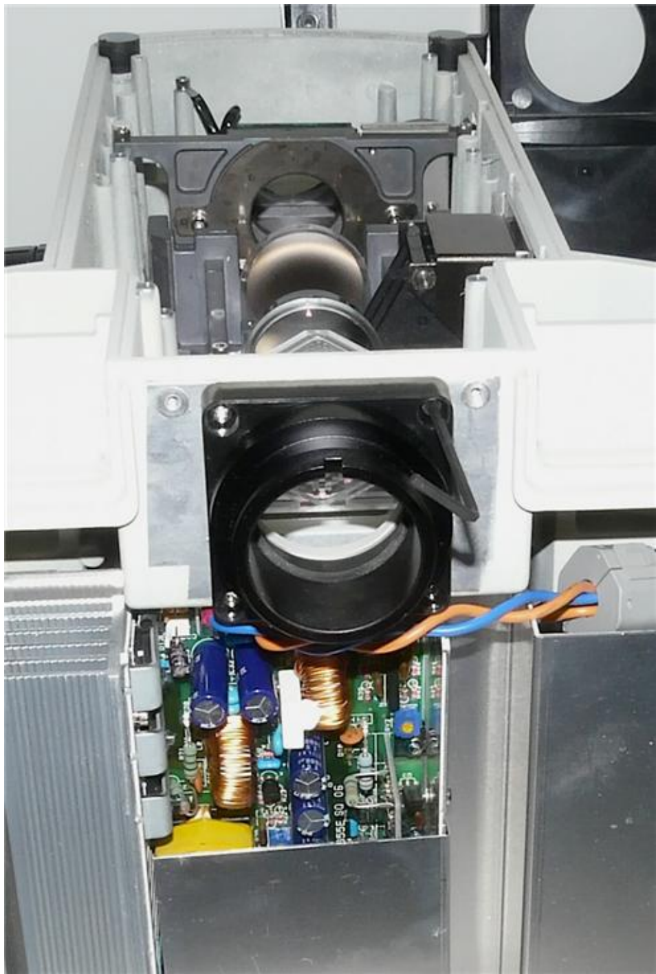
(1) Remove the original illuminator mount. Save the screws for the new adapter.
