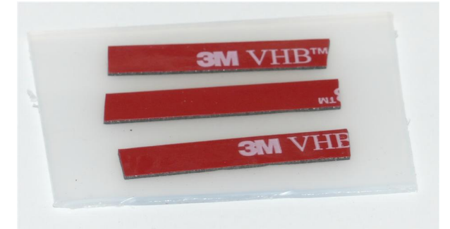
Tape to secure wires.
