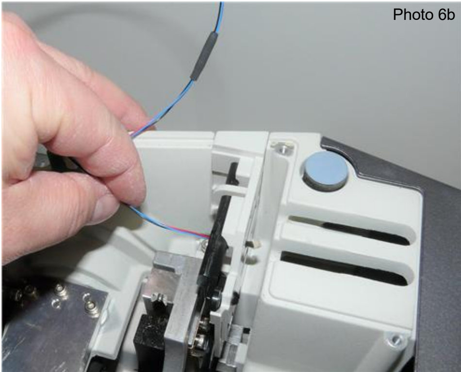
Route pot cable through the filter unit.
