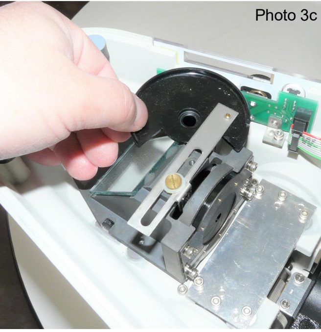
Slide the diaphragm control wheel away from the slot in the side of the microscope.
