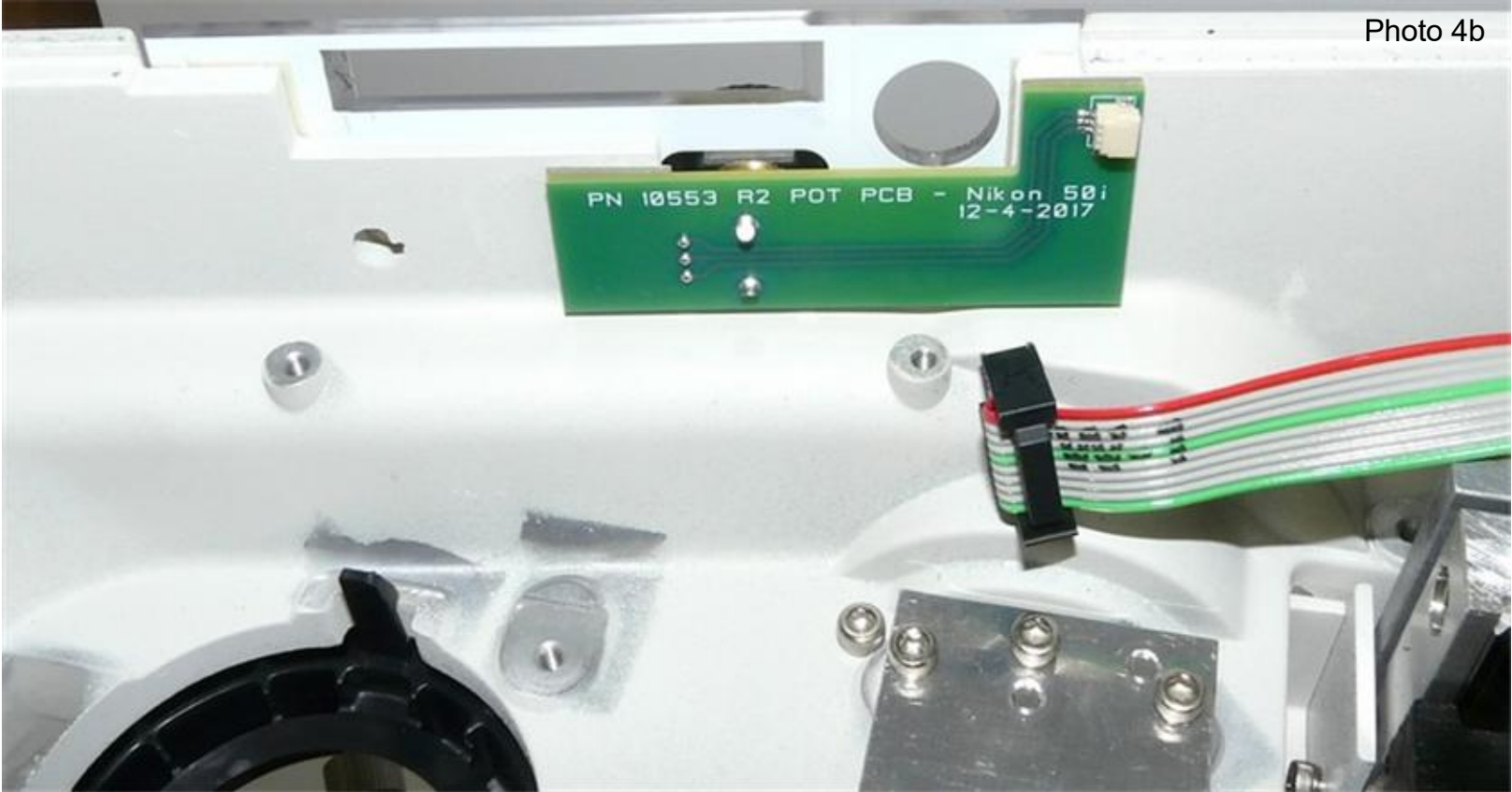
Press the tape surface against the inside of the microscope to secure the Nanodyne pot PCB. Be sure the shaft of the pot is centered in the hole in the microscope so it does not rub. Place the original knob on the new pot.
