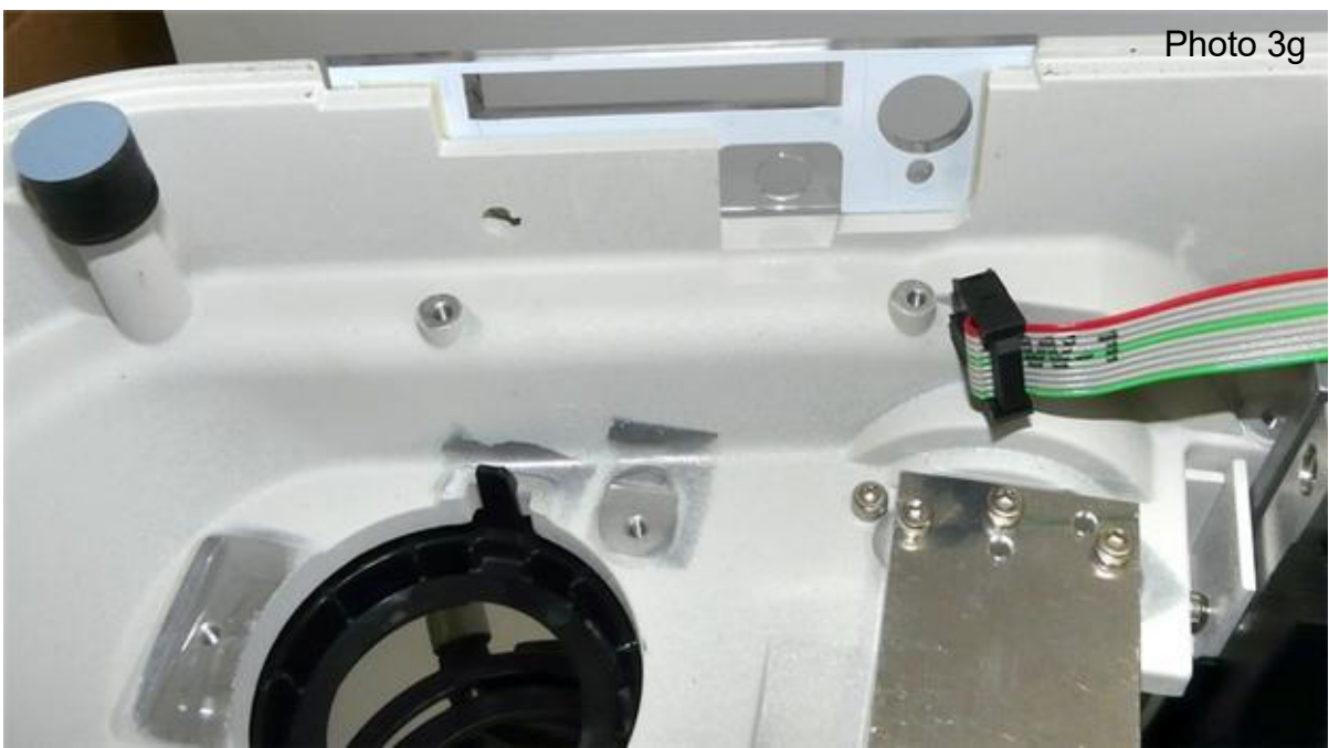
Original intensity control pot PCB removed.
