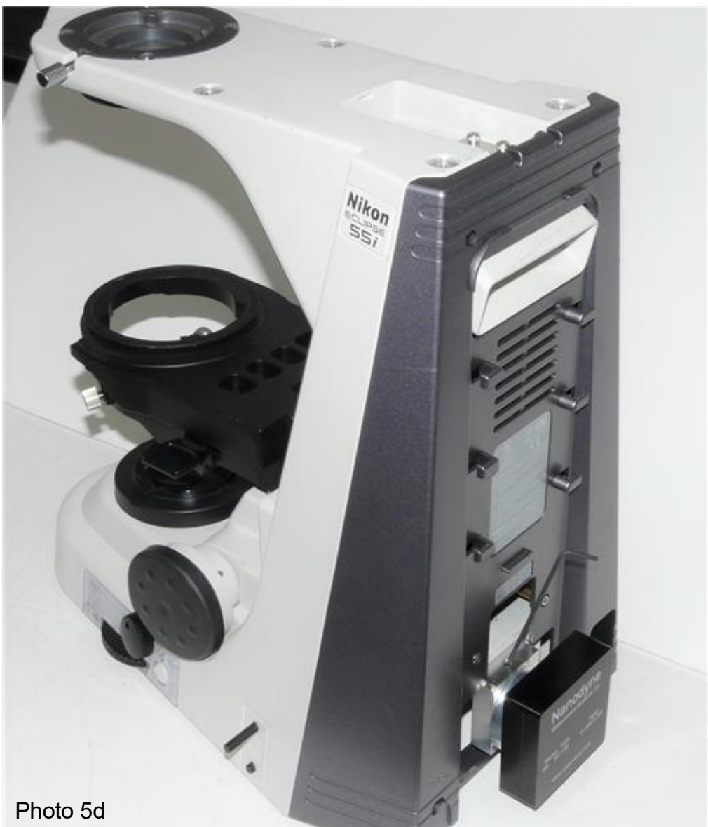
Reinstall the back cover and attach Nanodyne illuminator.
