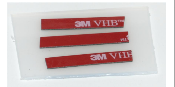
Tape to secure wires.
