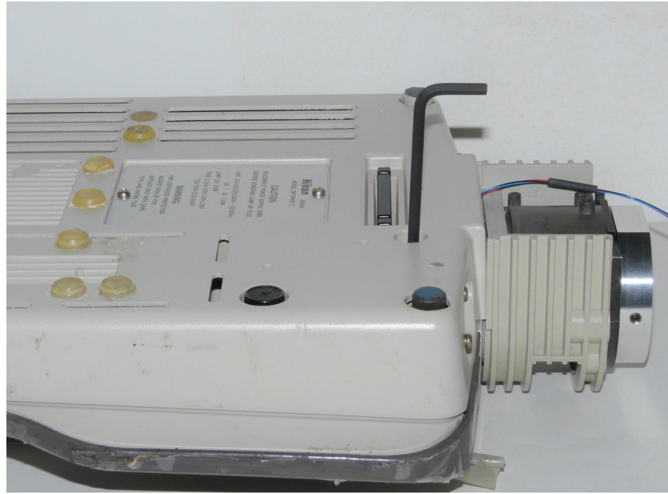
1. Replace the bottom cover. Secure with the original screws using the 4mm hex key.
