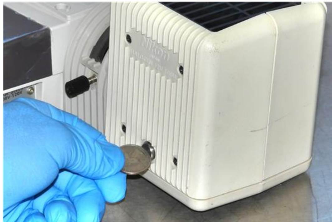
1. Remove cover from lamp housing by loosening the large stainless steel screw. A quarter fits the slot very well.
