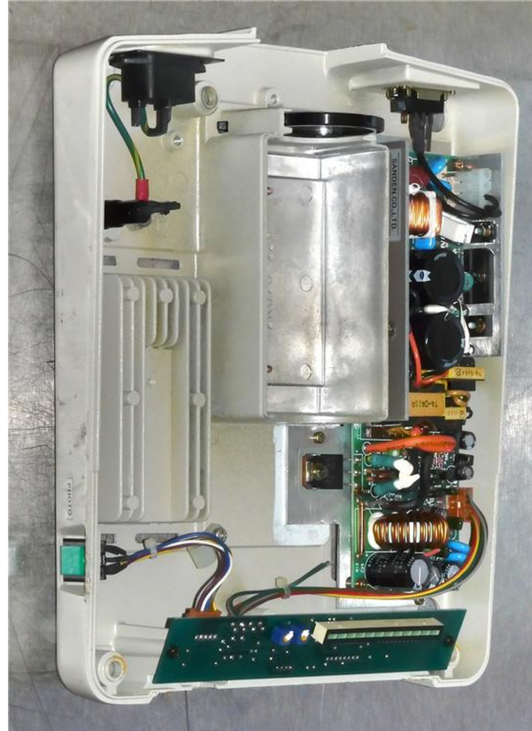
2. Bottom cover after removing unwanted items.
