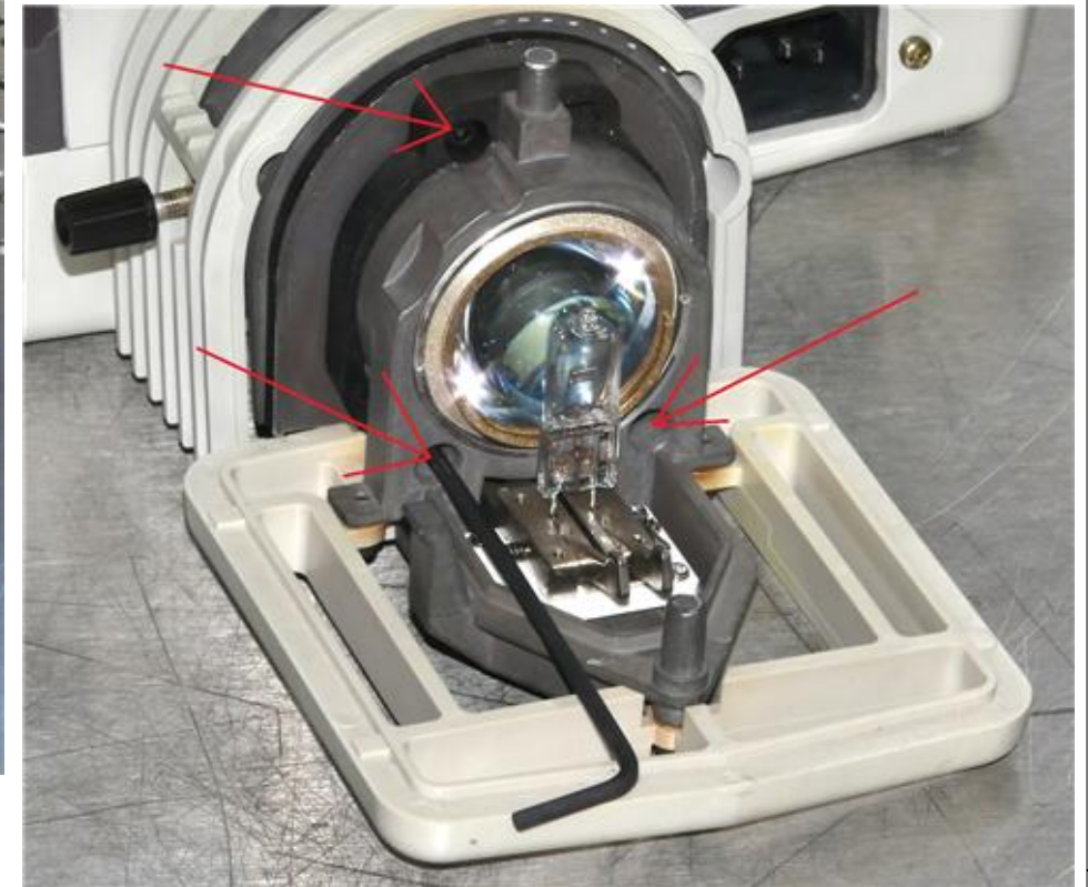
2. Remove the 3 screws holding lamp housing to microscope.
