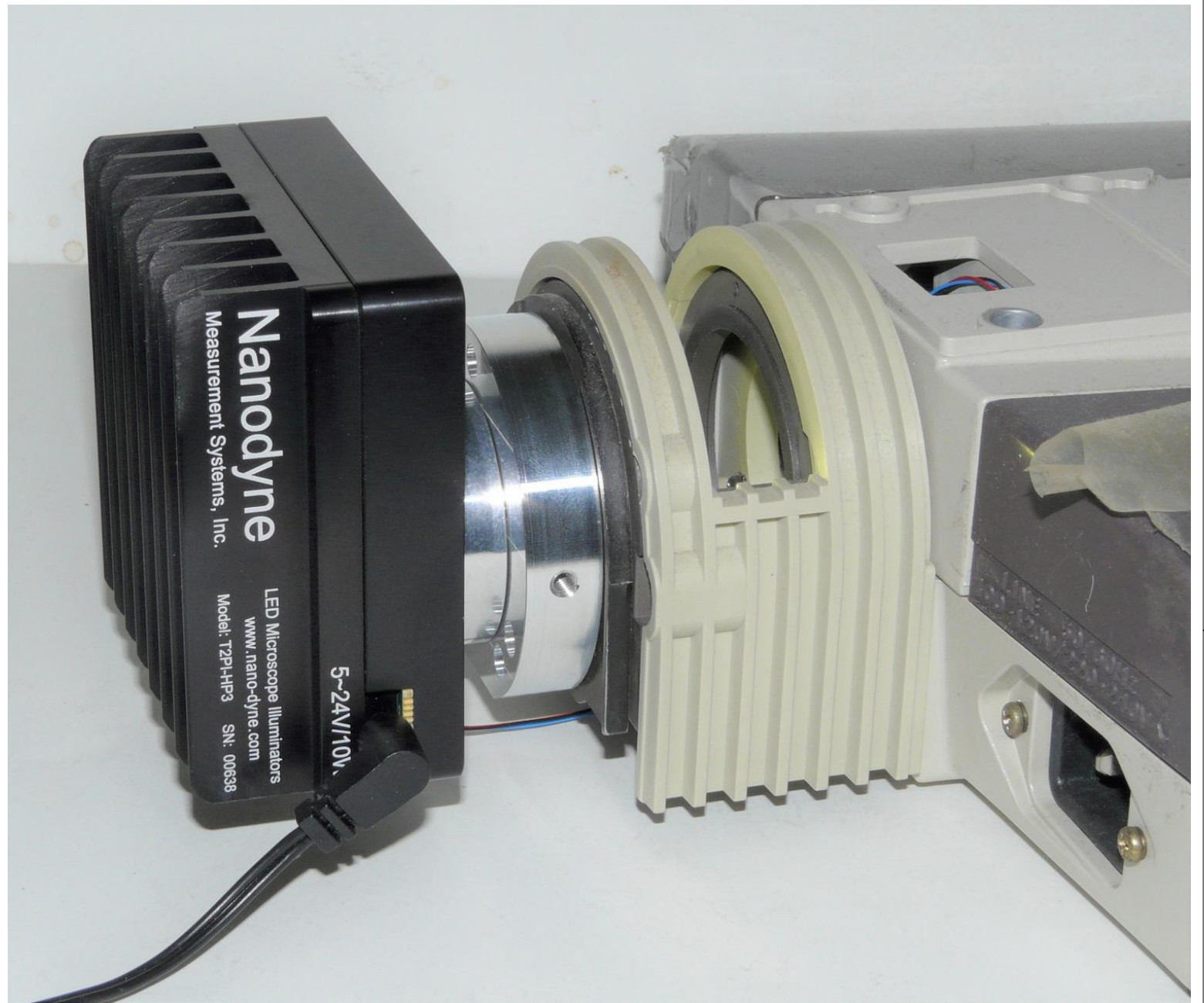
3. Connect the power supply cable to the illuminator as shown above.
