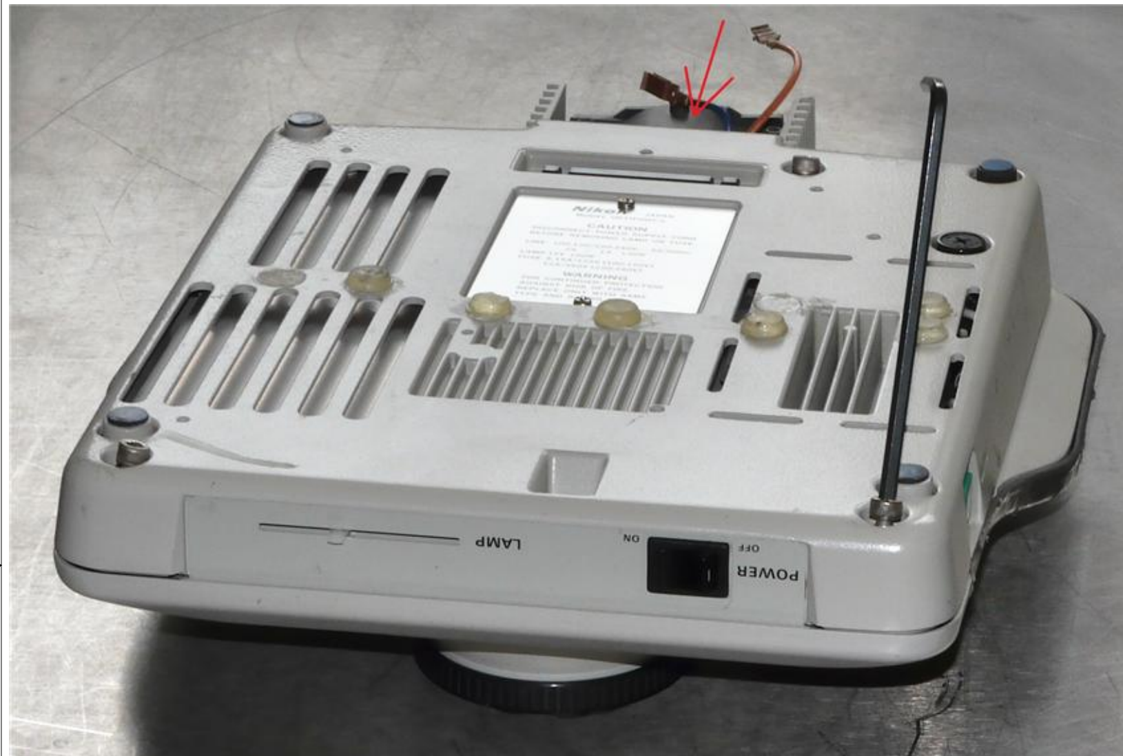
1. Use the 4mm hex key to remove the 3 socket head screws from the bottom of the base.
