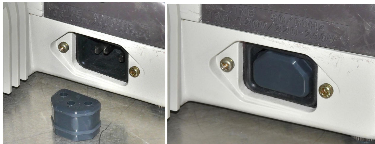
3. Install the silicone rubber blocking plug in the obsolete AC power receptacle.
