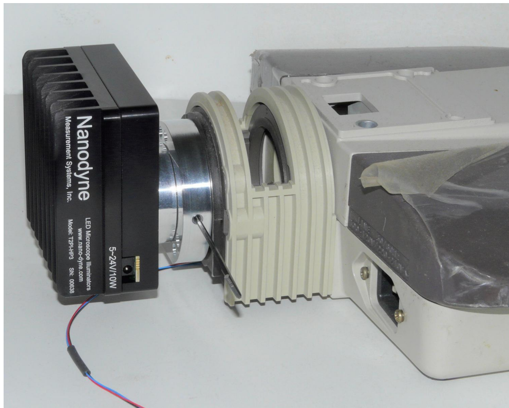
2. Insert the illuminator into the adapter and tighten the set screw with the 5/64 inch hex key as shown above.
