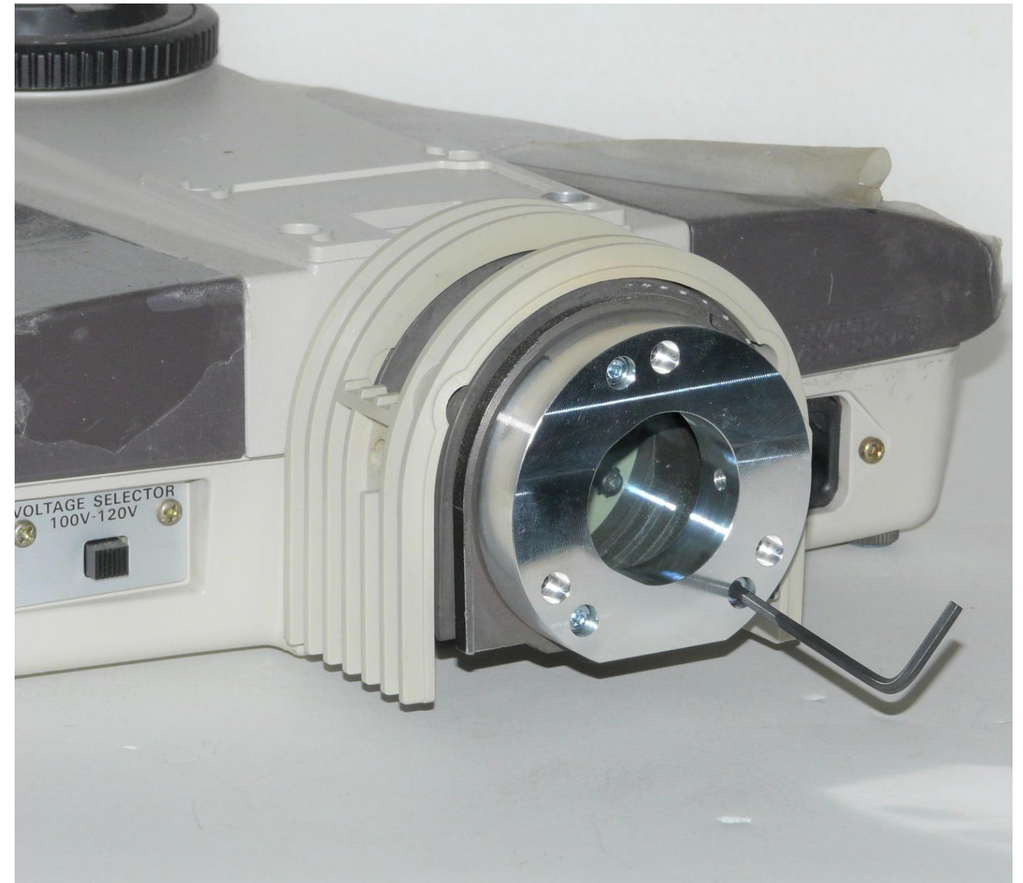
2. Attach the adapter ring using the three 12mm long M3 screws, using the 2.5mm hex key.
