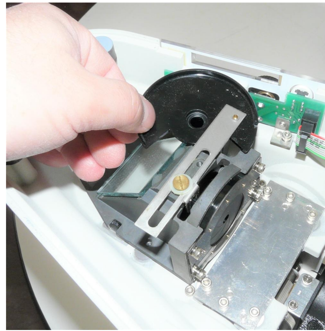
(3) Slide the diaphragm control wheel away from the slot in the side of the microscope.
