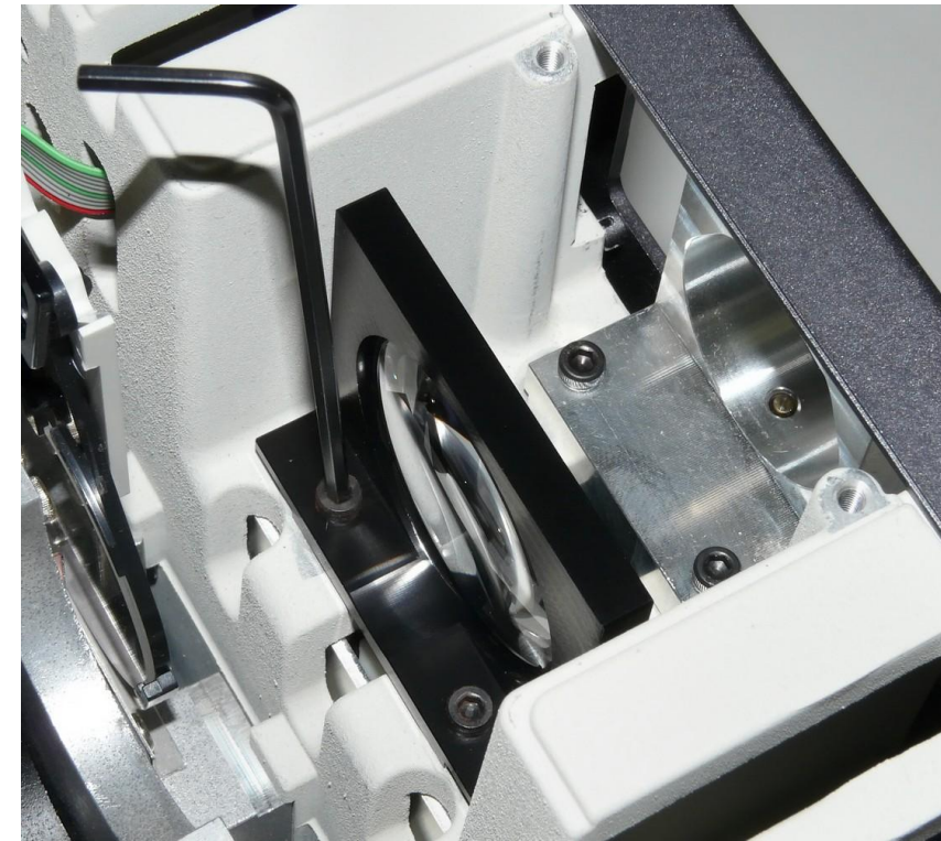
(3) Install the secondary lens assembly as shown above.
