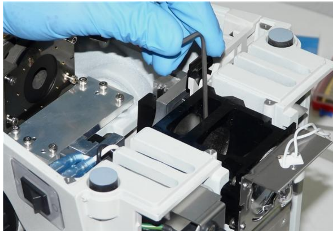
(2) Remove the 4 screws holding the collector lens assembly.
