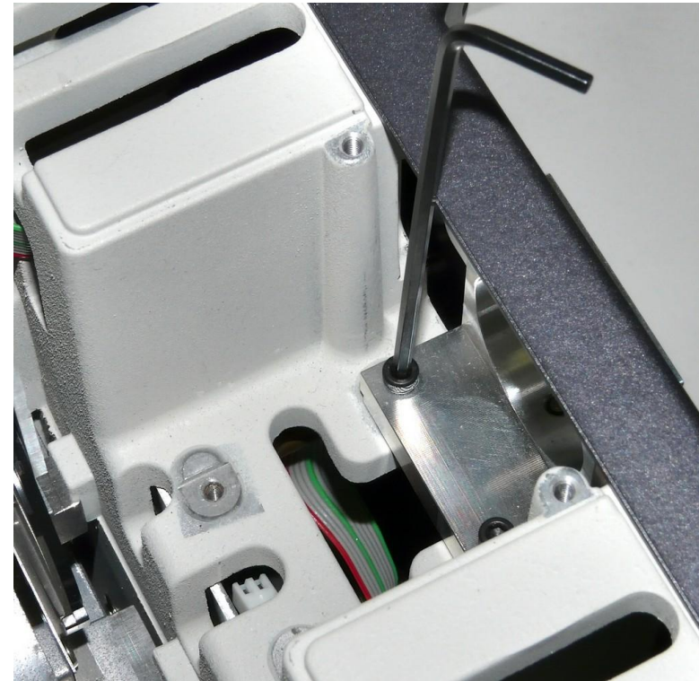
(2) Install the mounting adapter as shown above.
