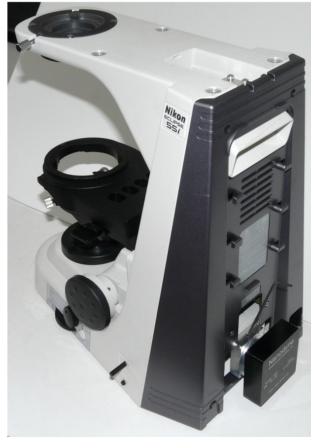
(4) Install the illuminator as shown at left.
