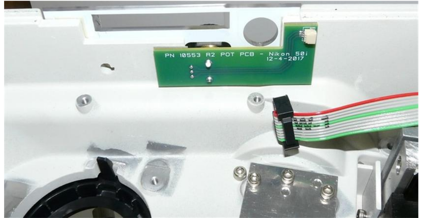
(2) Press the tape surface against the inside of the microscope to secure the Nanodyne pot PCB. Be sure the shaft of the pot is centered in the hole in the microscope so it does not rub. Place the original knob on the new pot.
