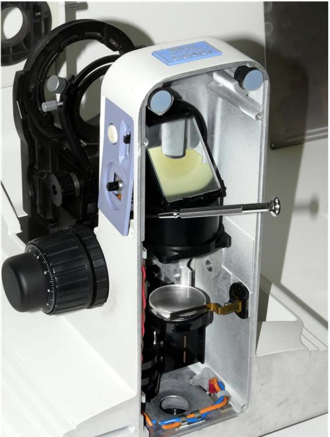
(2): Remove the plastic potentiometer plate as shown above. Push it out from the inside. Use a small screwdriver or similar tool if needed.
