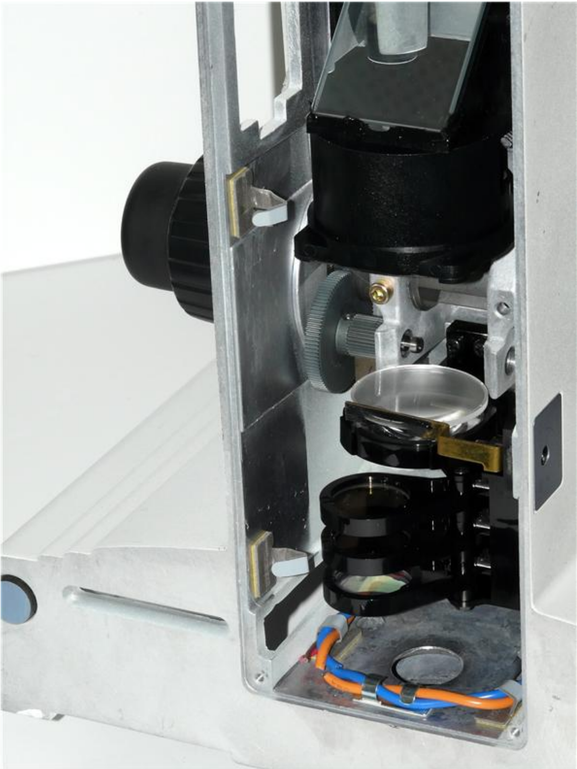
(1): Disconnect and remove the wires that go from the old pot plate to the old power supply.
