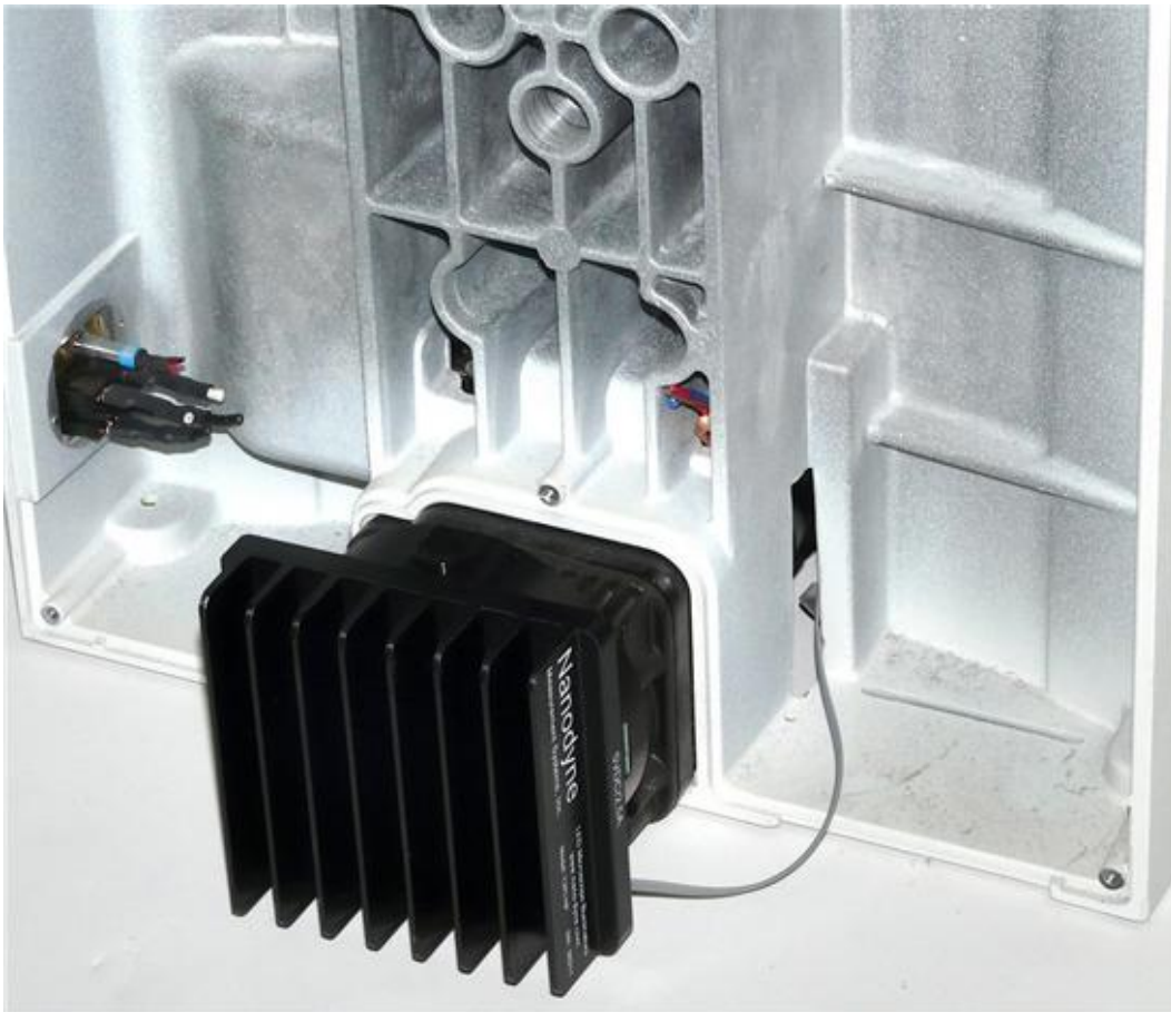
(3): Connect the pot cable to the socket on the bottom of the illuminator.
