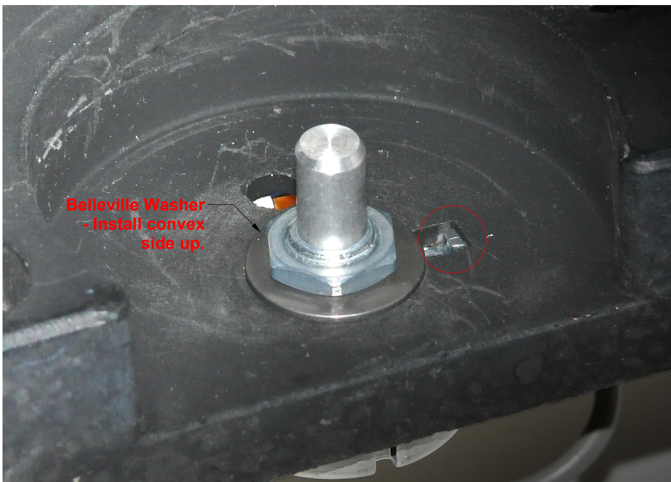
(3) Install the Nanodyne pot as shown. The Anti-Rotate tab goes in the slot in the microscope (red circle). With an 11mm socket, snug the nut finger tight, then using the handle for the socket, tighten at least 1/4 turn, but less than 1/2 turn.
