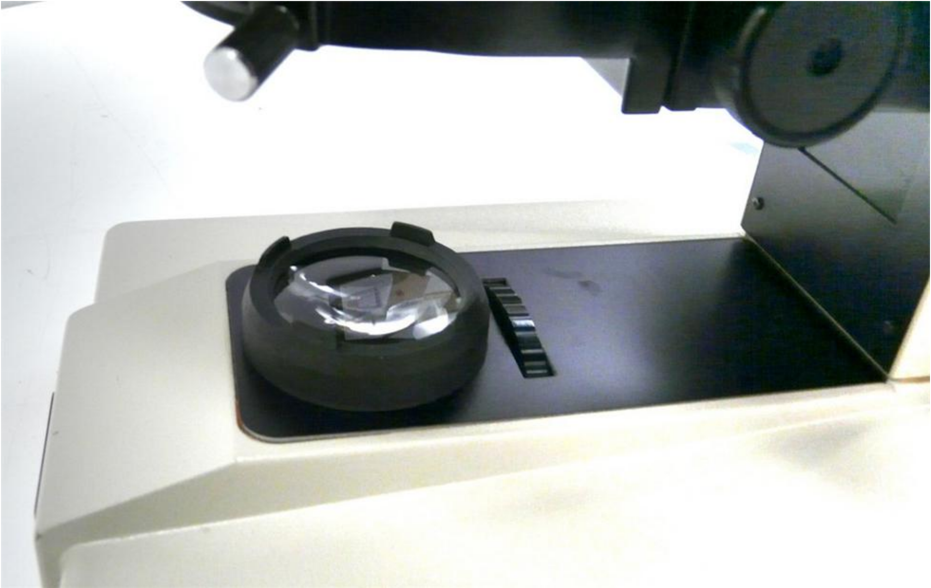
(1) Replace the lens and lens holder.
