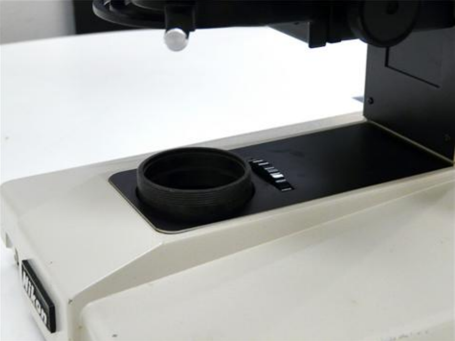
(2) Unscrew and remove the black ring and lens.
