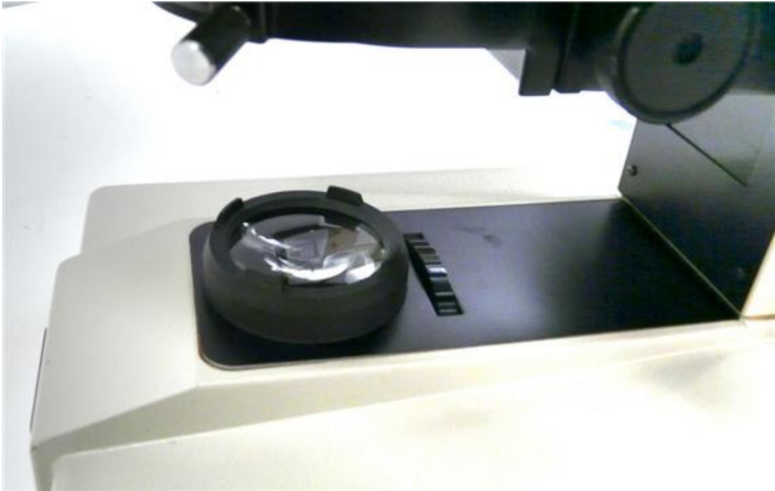
(1) The black ring around the lens must be removed to open the microscope.
