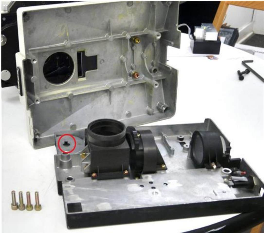
(2) Bottom cover removed. Note that the pot will still be in place at the red circle, and the electronics were stripped out before we got it.
