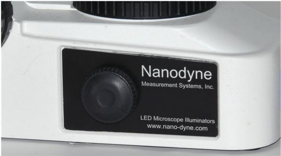
(6): Put the original knob on the new potentiometer shaft. Tighten with the 1.5mm hex key provided. For better appearance, back off the set screw so it fits on the round part of the shaft, rather than the flat, for a closer fit to the plate.
