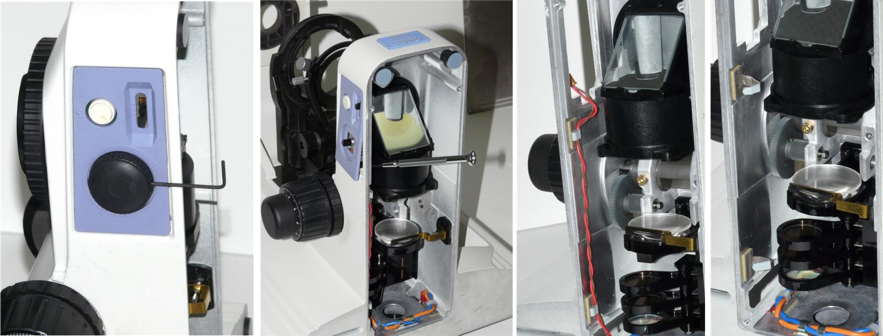
(3) Remove the pot cable as shown above. Cut the far end as shown and discard the cable.
