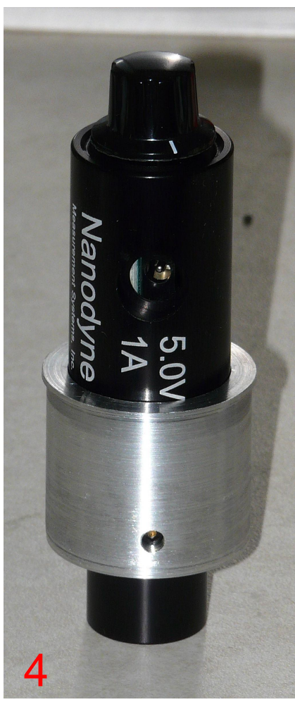
3. Nanodyne illuminator inserted as far as possible into the adapter.
