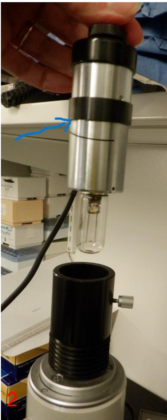
3. Nanodyne illuminator inserted as far as possible into the adapter.
