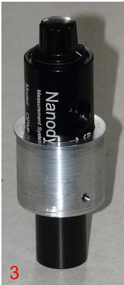
3. Nanodyne illuminator inserted as far as possible into the adapter.
