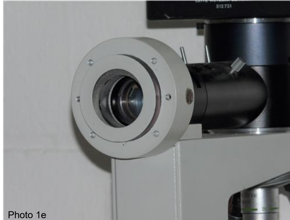
5. Microscope port after removing the original mounting ring.
