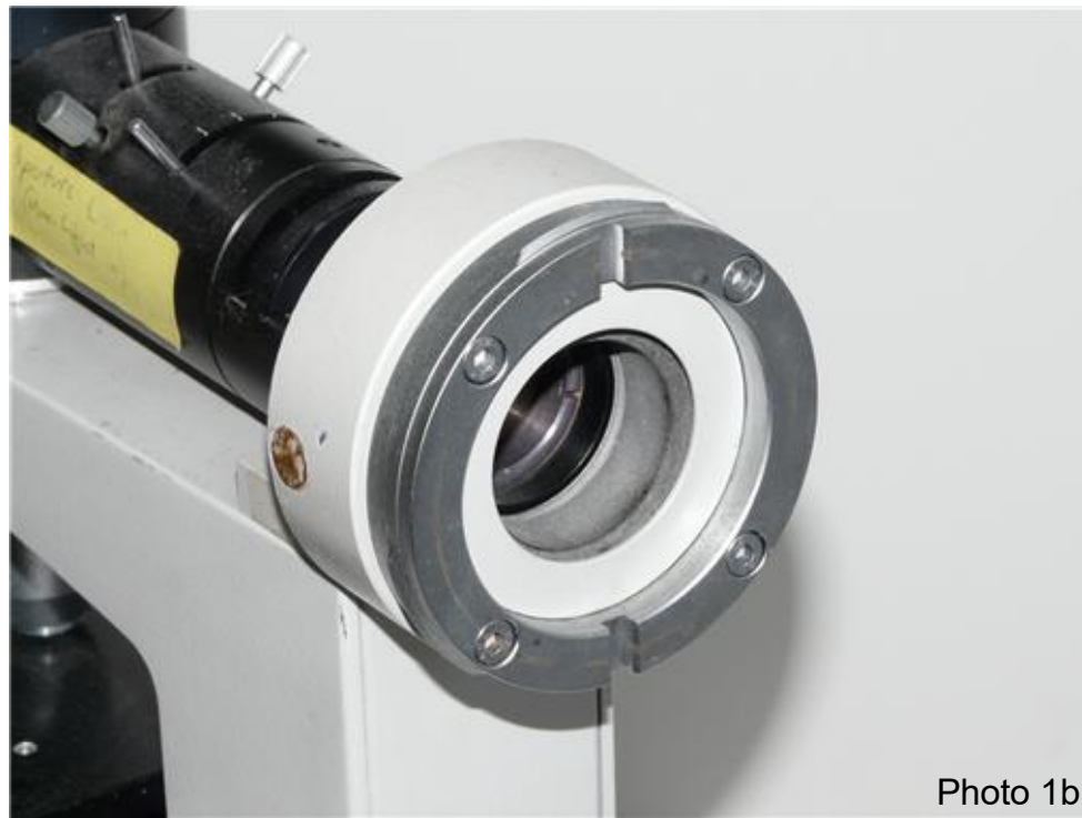
2. Original lamp housing removed.
