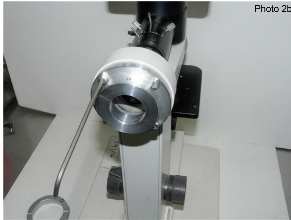
2. Secure the Nanodyne adapter to the microscope with the original screws (M4 x 0.7 x 16mm).
