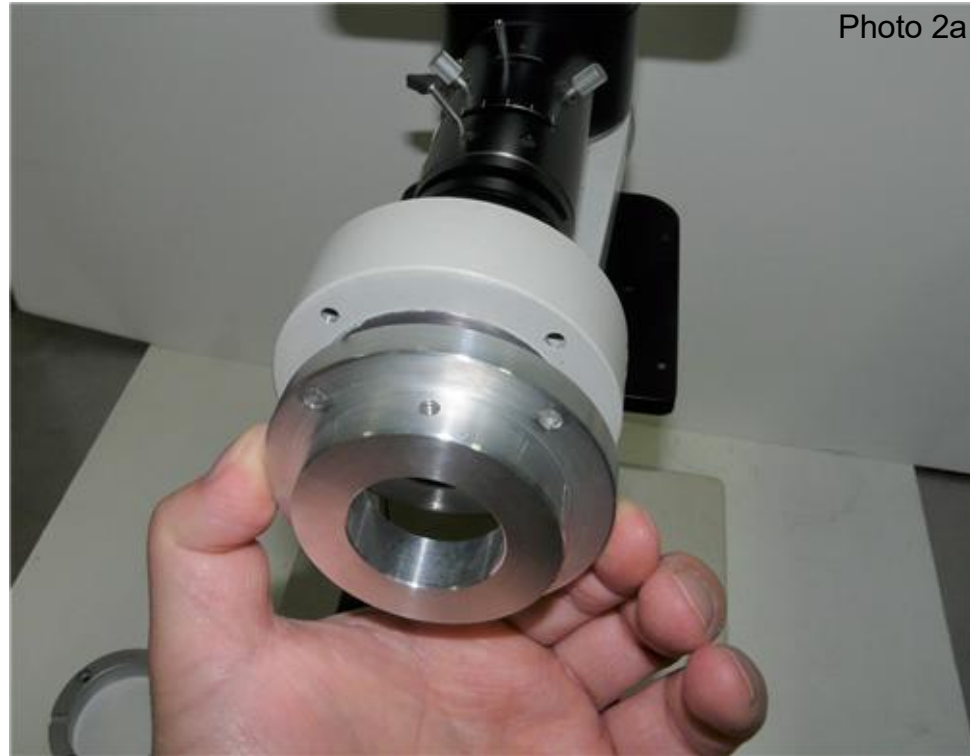
1. Align the Nanodyne adapter with the microscope.
