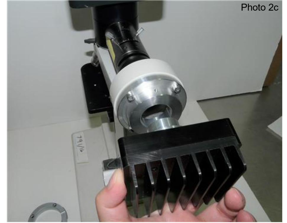
3. Insert the Nanodyne illuminator into the Nanodyne adapter
