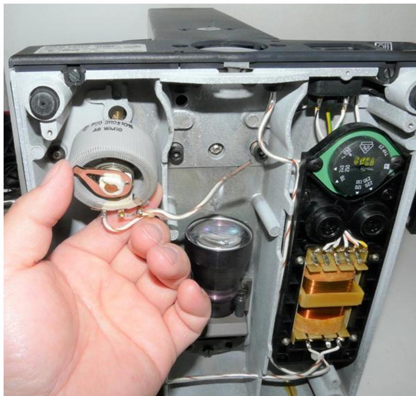
(5) Remove OEM potentiometer and all wire connections to the AC power receptacle.
