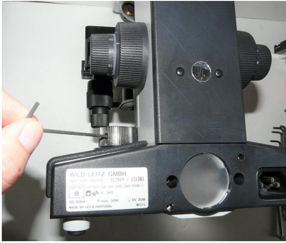
(4) Loosen the set screw using the 5/64 in hex key provided.
