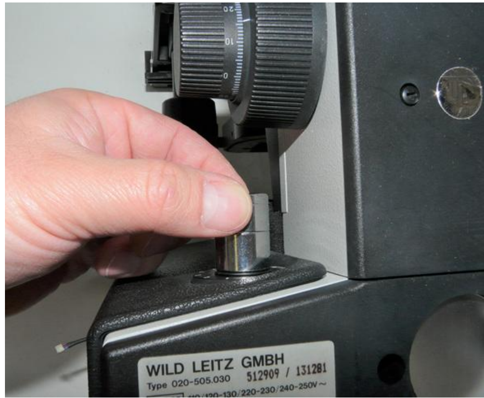
(3) Tighten the nut holding the adjustment pot using a 13mm hex socket. You can use a wrench if desired.
