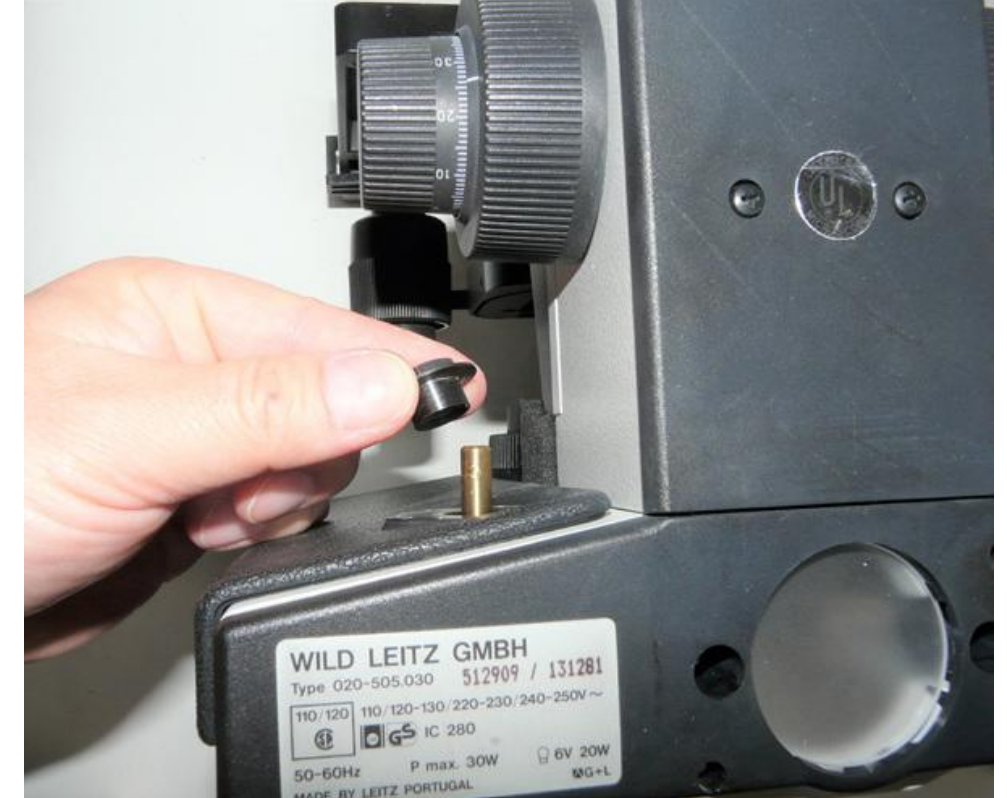
(3) Remove the nut and washer, and keep it for later.
