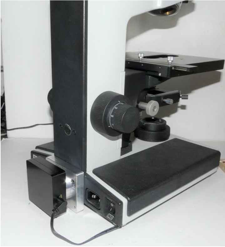
(4) Plug in power cable to the illuminator.
