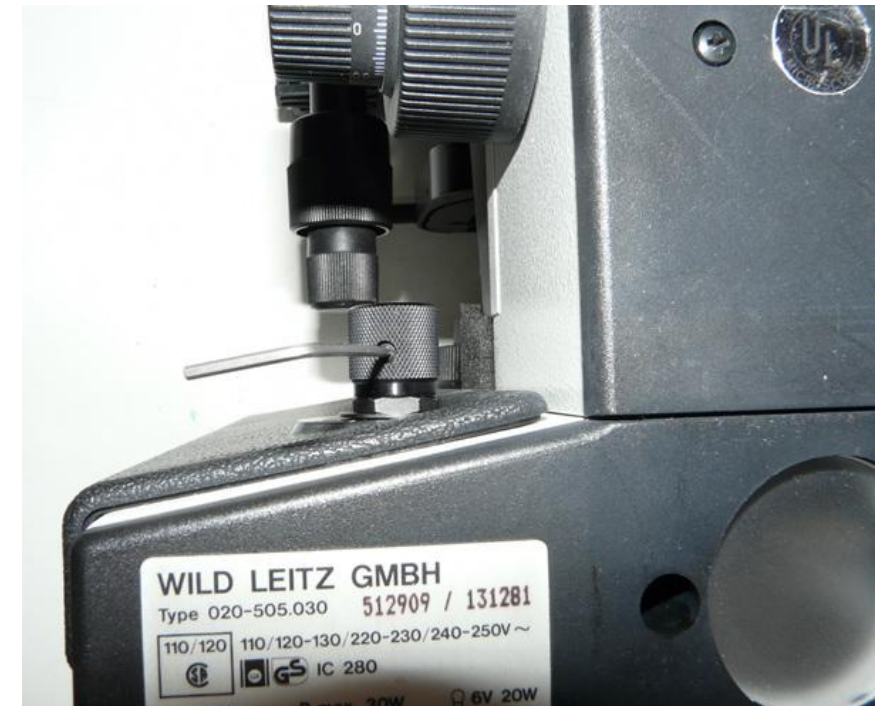
(4) Install the new knob provided using the 1/16 in hex key.
