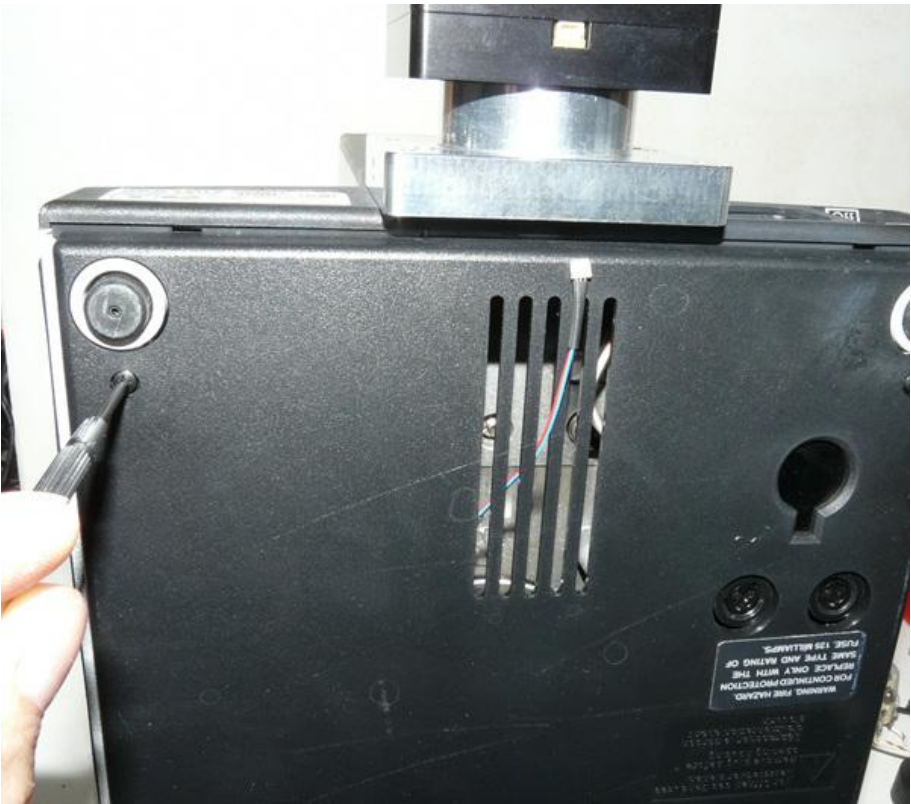
(1) Tighten the 4 original screws saved.
