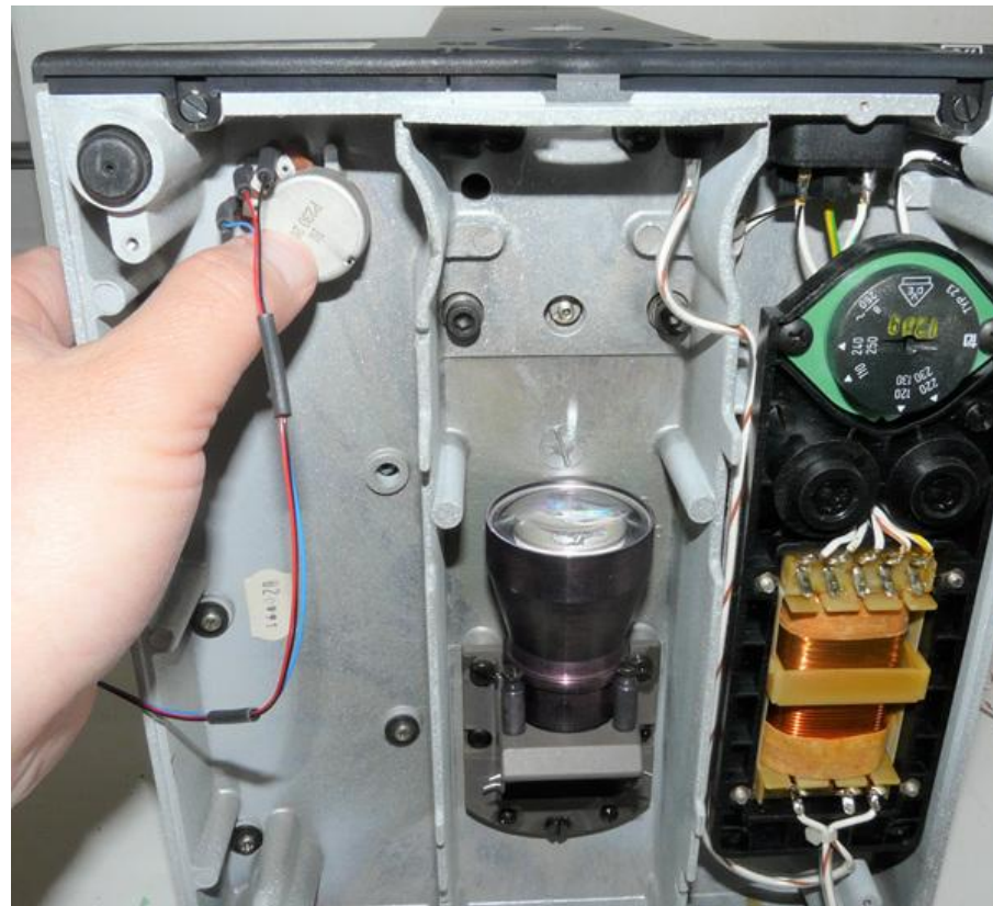
(2) Secure the new pot in place with the original nut and washer.
