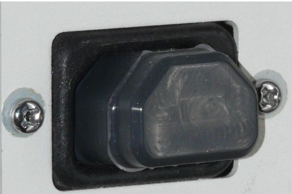
(5) Insert PN 10736 rubber plug to block now-obsolete AC power receptacle.
