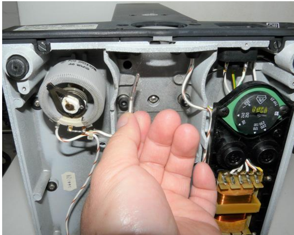
(4) Disconnect the OEM pot cable.
