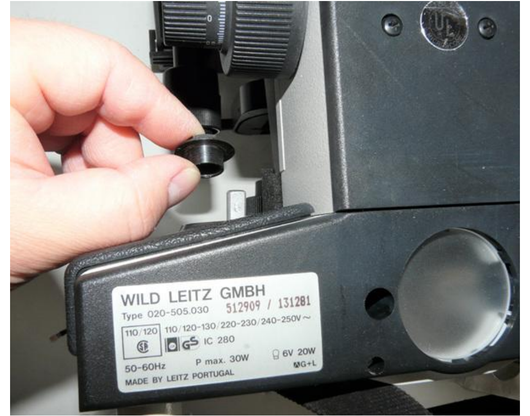
(2) Secure the new pot in place with the original nut and washer.
