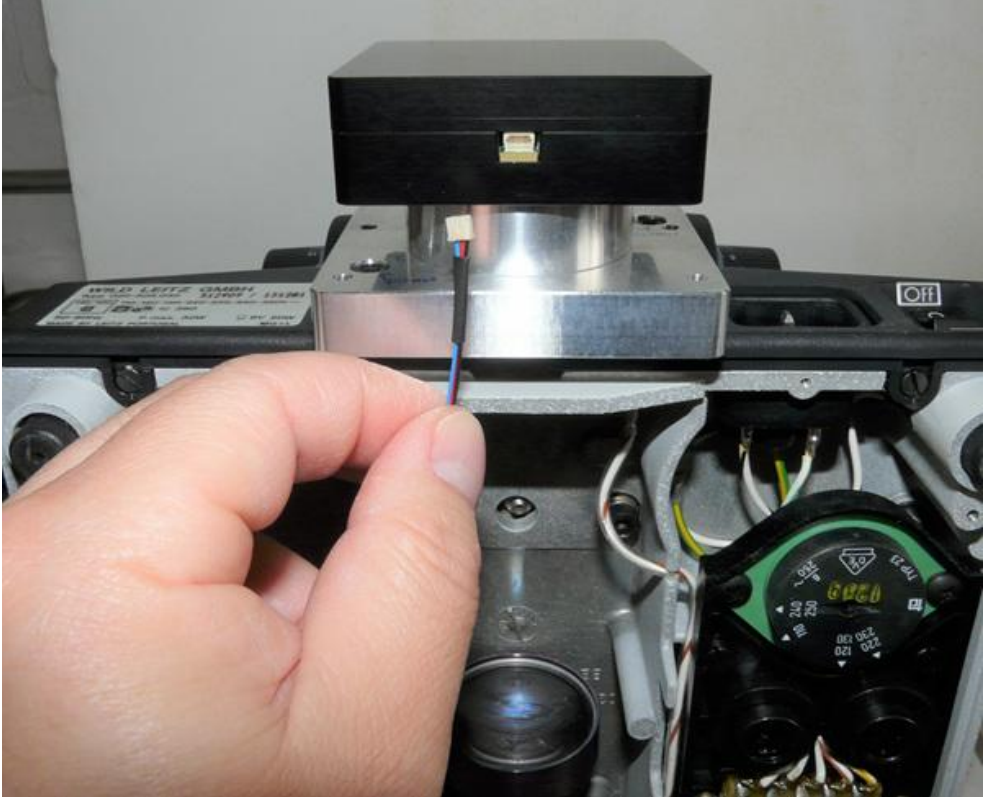
(5) Put the pot cable through the slit and replace the bottom cover.
