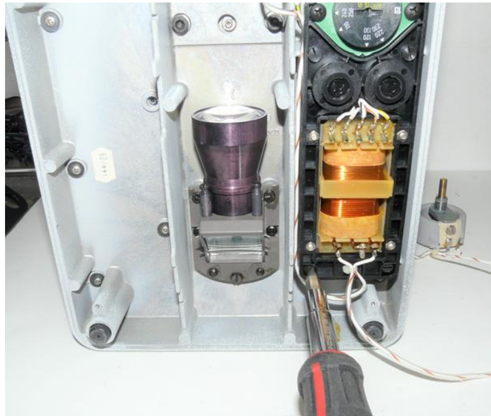
(1) Remove now-obsolete old transformer if desired.
