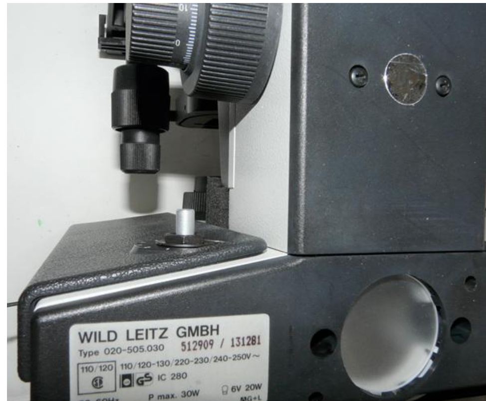
(3) Tighten the nut holding the adjustment pot using a 13mm hex socket. You can use a wrench if desired.
