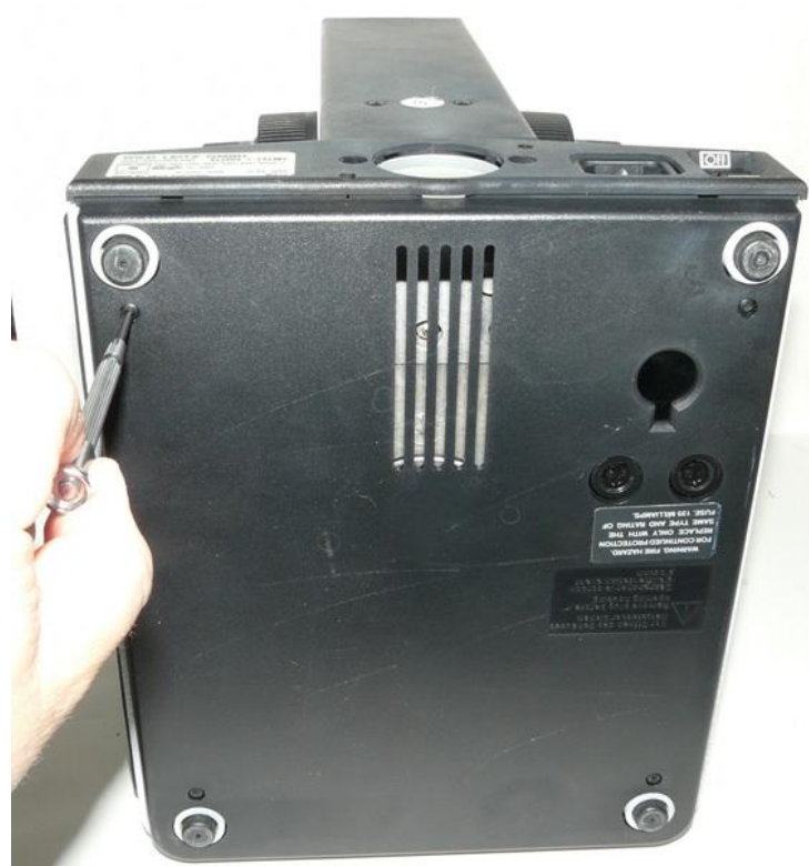
(2) Remove the 4 screws holding bottom cover using screw driver and open the bottom cover. Keep the screws for later.
