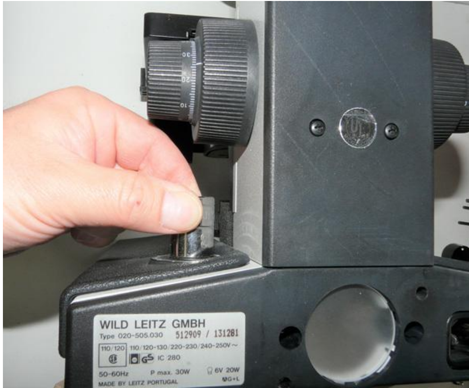
(1) Unscrew the nut holding the OEM pot using a 13mm hex socket.
