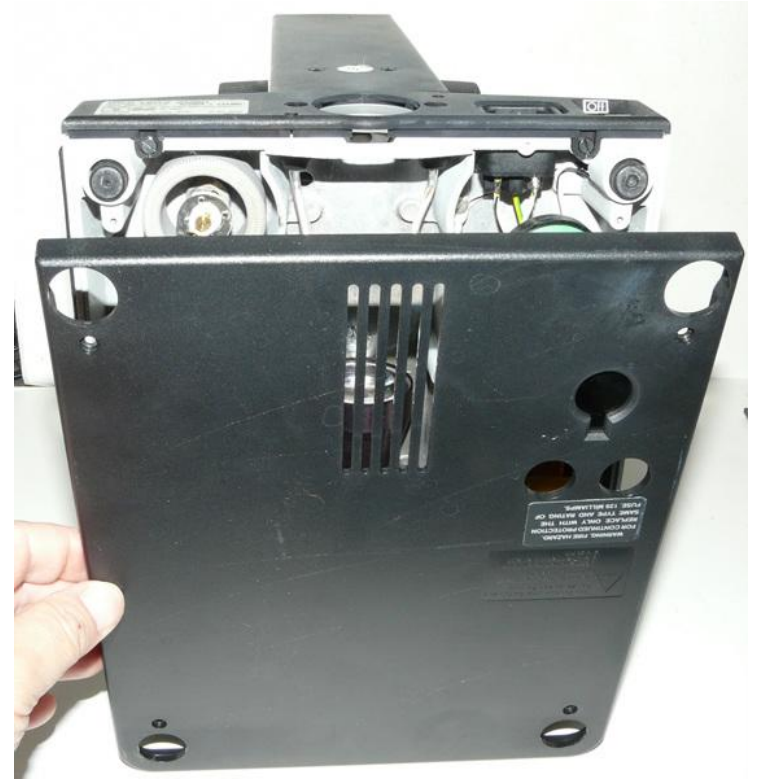
(2) Remove the 4 screws holding bottom cover using screw driver and open the bottom cover. Keep the screws for later.
