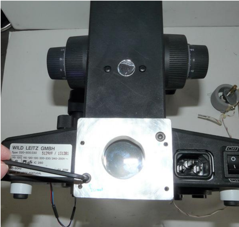
(1) Install Nanodyne adapter with the two M4 screws provided.
