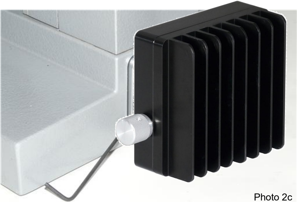
(3) Insert the Nanodyne illuminator and secure by tightening the set screw. Note that the set screw on the current adapter is at the top rather than the side.
