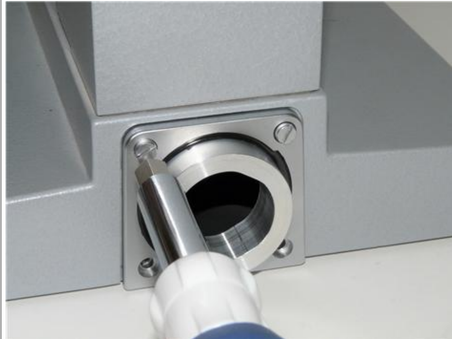
(1) Attach the Nanodyne adapter using the original screws. (Photo is of a prototype test adapter)
