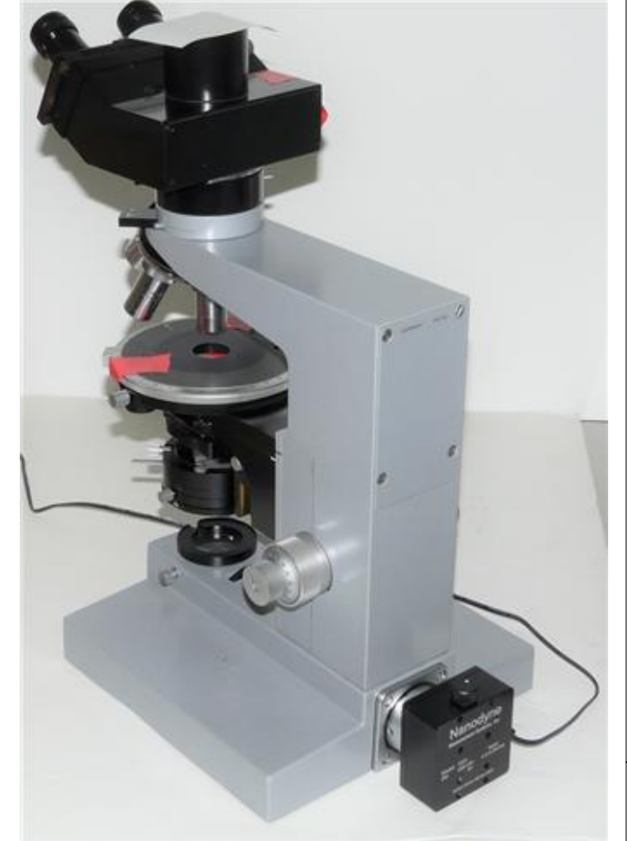
(4) Connect the power supply and it is ready to use. The unit is fully off when the adjustment knob is turned counter clock wise. There may or may not be a click to indicate "off". Do not force it.
