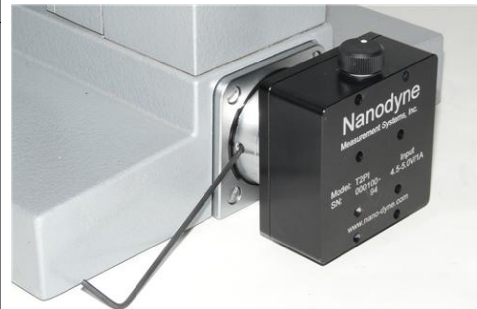
(1) Attach the Nanodyne adapter using the original screws. (Photo is of a prototype test adapter)
