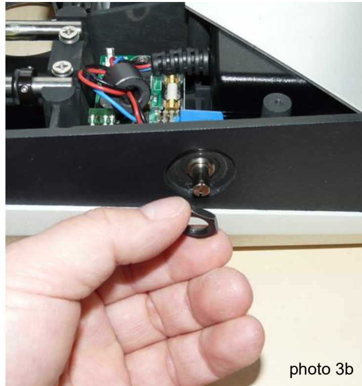
(1) Unscrew and remove the OEM nut. Keep the nut for later installation.
