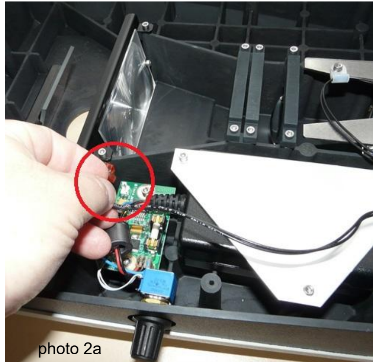
(1) Disconnect the original lamp.
