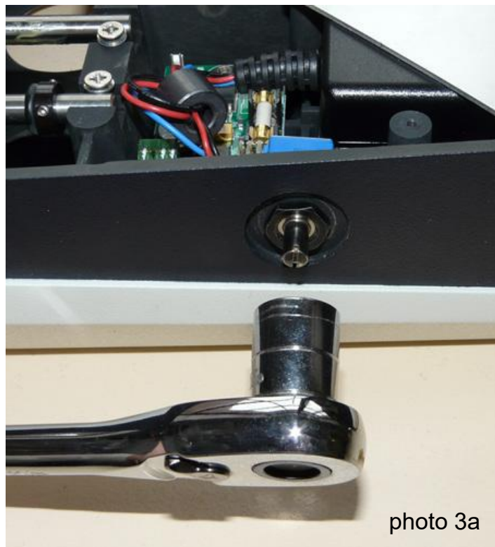
(1) Unscrew and remove the OEM nut. Keep the nut for later installation.
