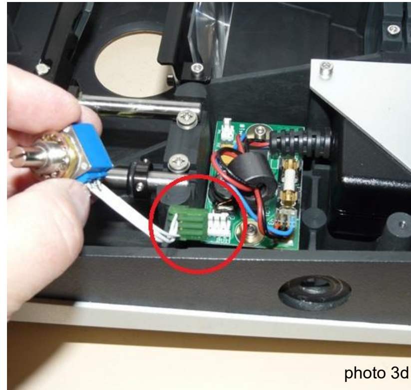
(2) Remove and disconnect the OEM potentiometer.
