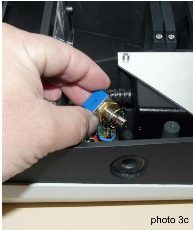
(2) Remove and disconnect the OEM potentiometer.
