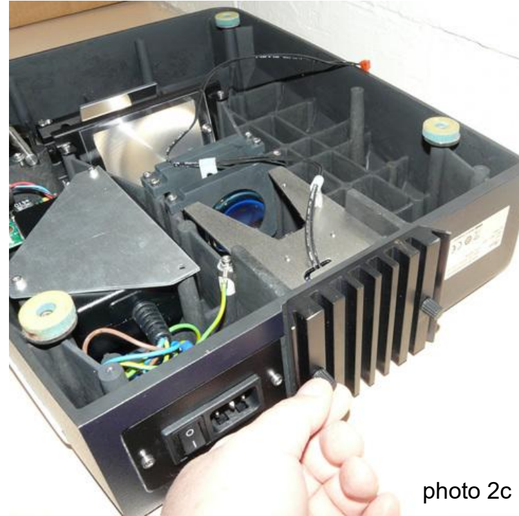
(3) Loosen the screws holding original lamp house.
