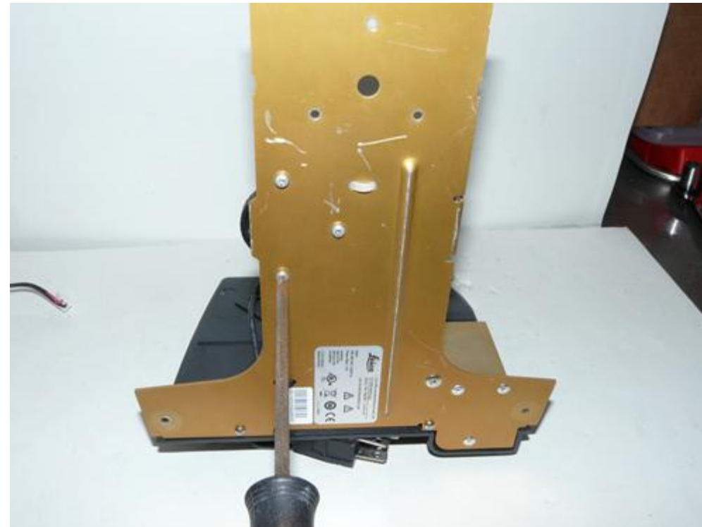
Remove 3 screws holding intensity adjustment pot housing.
