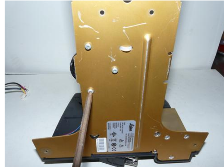
Re-install the potentiometer mounting bracket using original screws.
