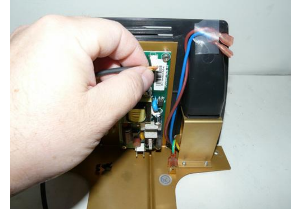
Unplug intensity adjustment cable from the original PCB.
