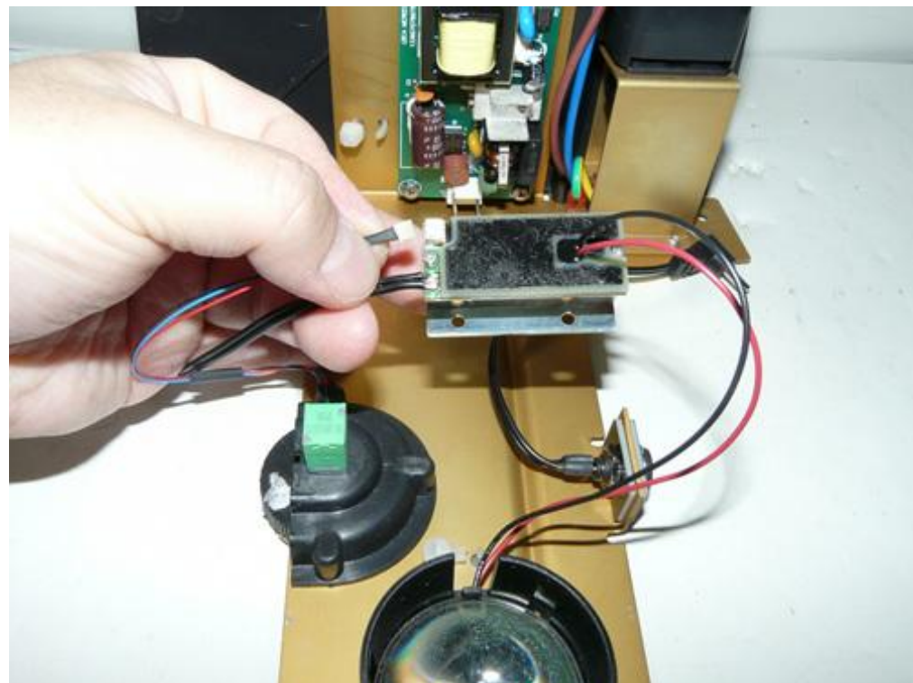
Connect a new pot cable to the Nanodyne illuminator assembly.
