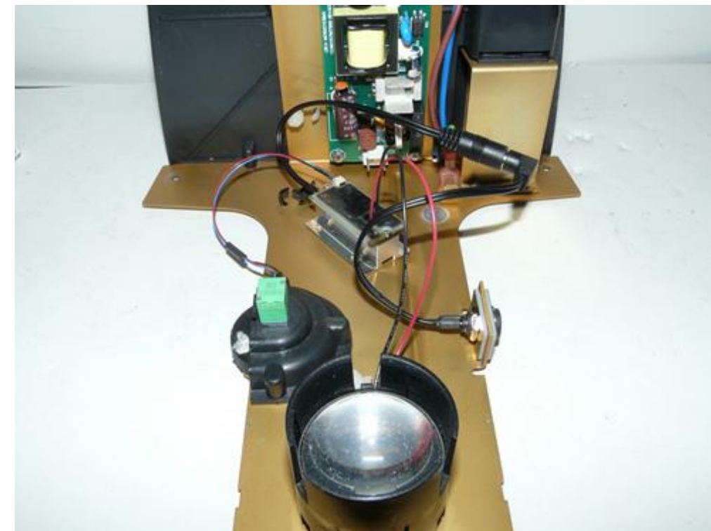
Organize pot cable and wires, fix PCB assembly using 3M VHB tapes provided.
