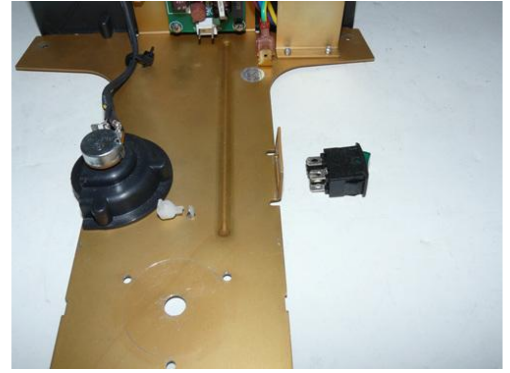
Depress the plastic clips on each side of the AC power switch and push it out.
