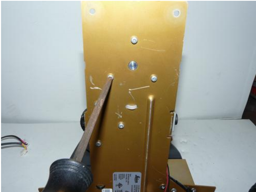
Re-install the original condensor lens assembly on the Nanodyne LED holder using original screws.
