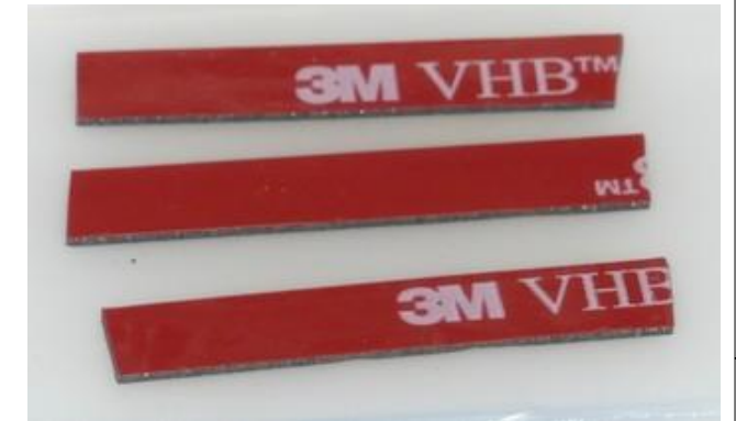
3M VHB Tape to secure wires.
