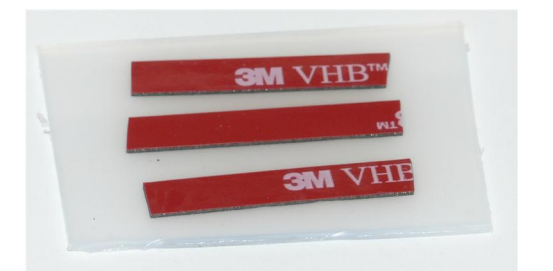
Tape to secure wires.
