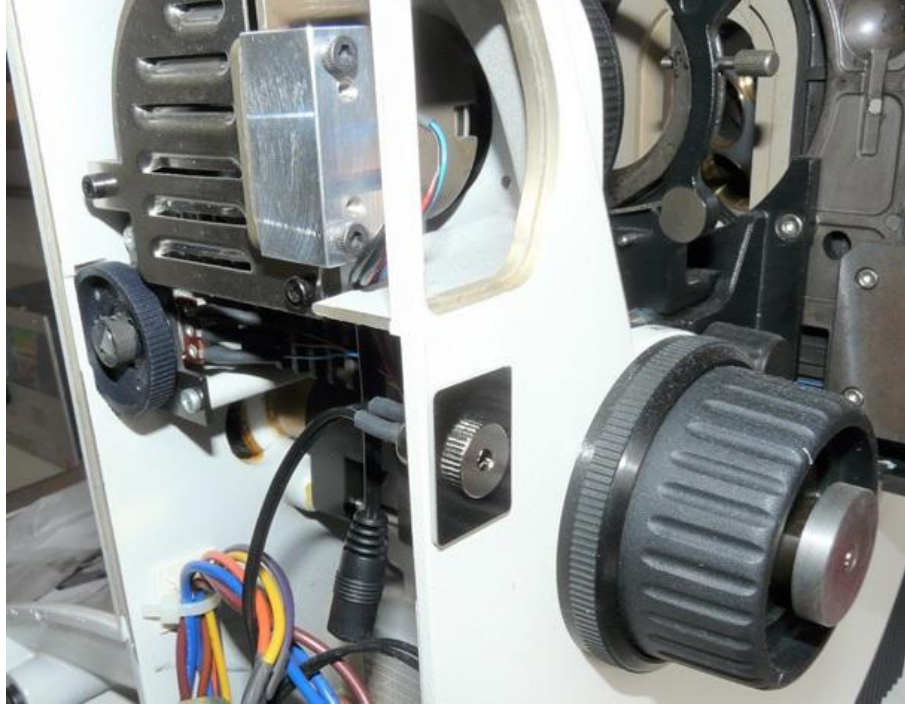
Line up the power plate (on the inside), and another plate (on the outside) with the AC power switch hole on the microscope frame. Then thread the nut onto the silver metal power jack and tighten it by hand. Verify that both plates are properly aligned with the nut finger tight. Then finish tightening with a wrench, just enough to secure them. Don't over-do it.
