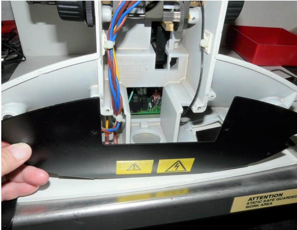
Unscrew and remove the bottom cover-2.
