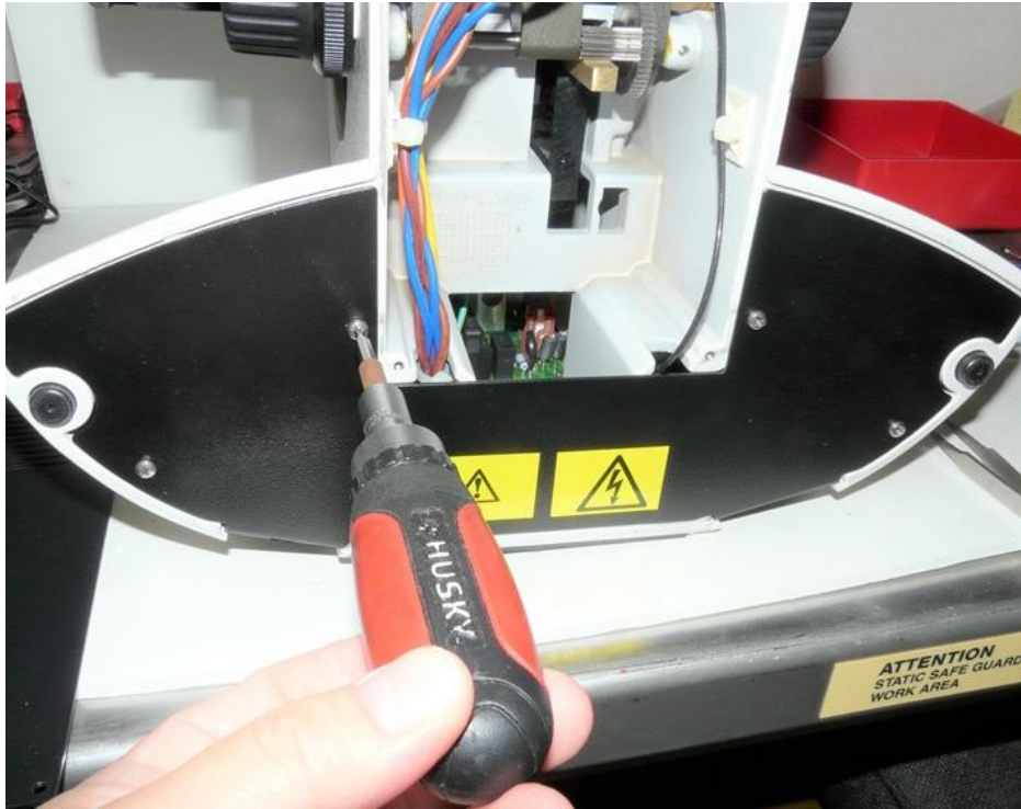
Unscrew and remove the bottom cover-2.
