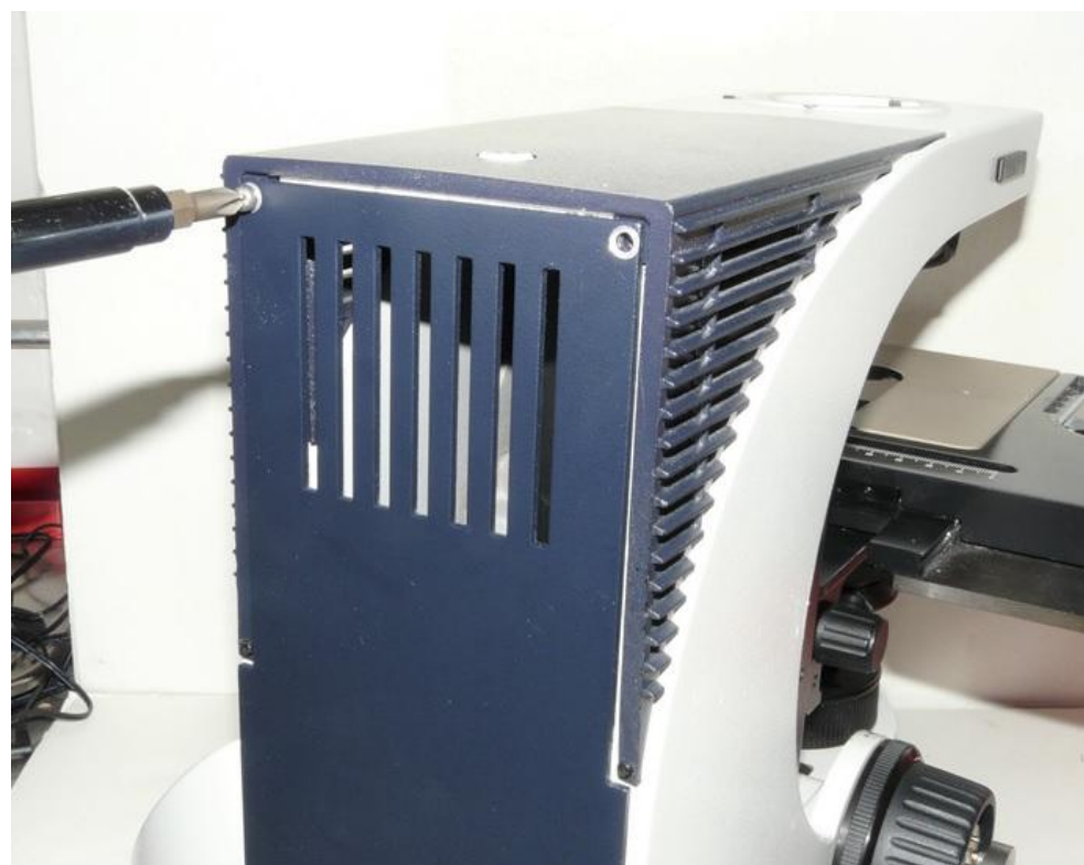
Reinstall the back cover.
