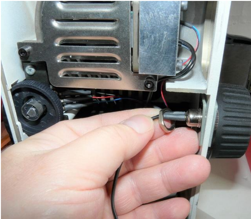
Line up the power plate (on the inside), and another plate (on the outside) with the AC power switch hole on the microscope frame. Then thread the nut onto the silver metal power jack and tighten it by hand. Verify that both plates are properly aligned with the nut finger tight. Then finish tightening with a wrench, just enough to secure them. Don't over-do it.
