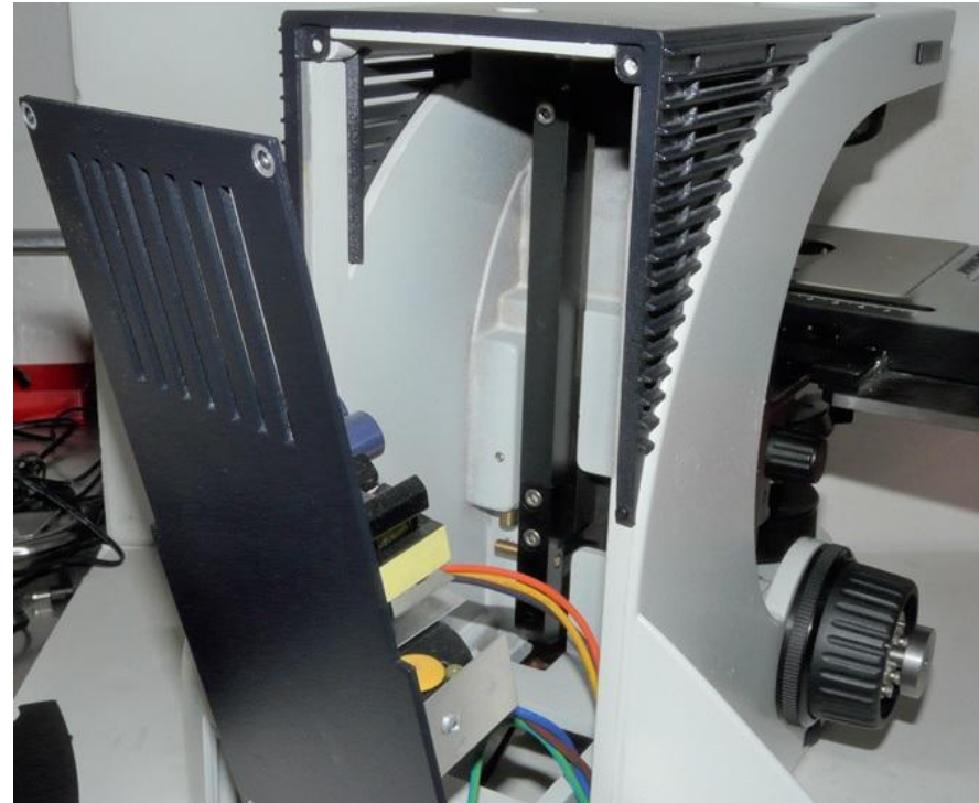
Unscrew and remove the back cover.
