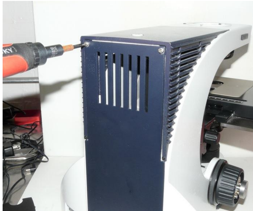
Flip the microscope to face back cover.
