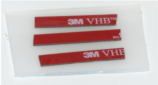
Tape to secure wires.
