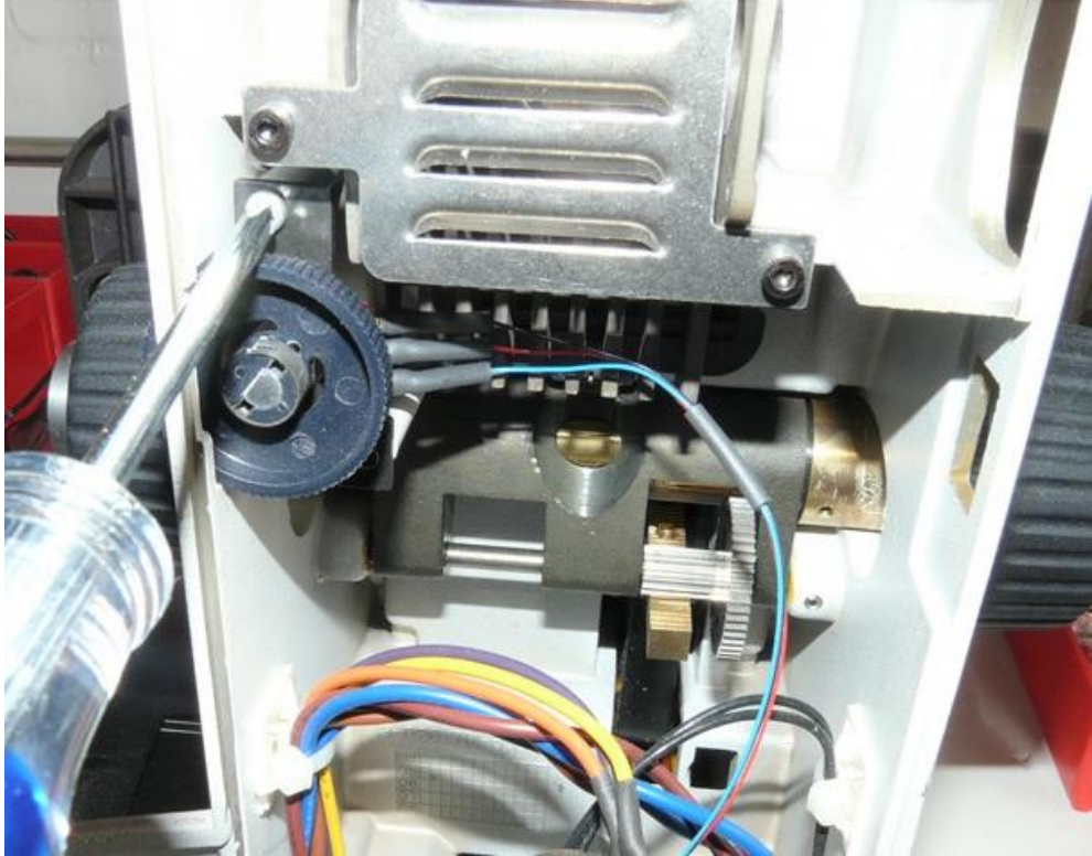
Re-install the potentiometer mounting bracket using original screws.
