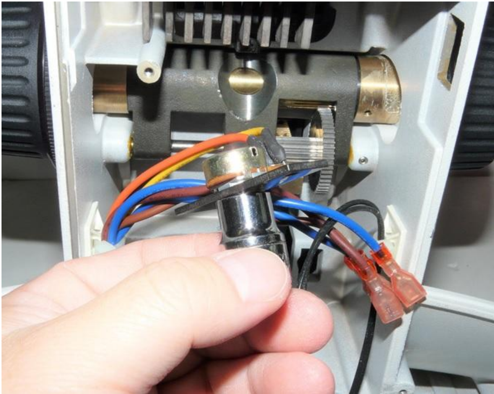
Loosen the nut using a wrench or socket. Unscrew to remove the old potentiometer.
