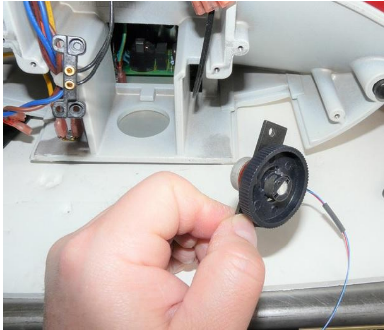
Re-install the original knob.
