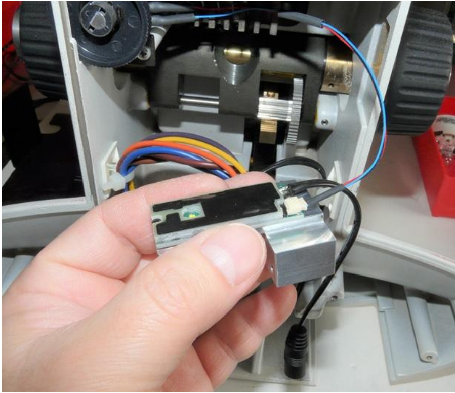
Connect a new pot cable to the Nanodyne illuminator assembly.
