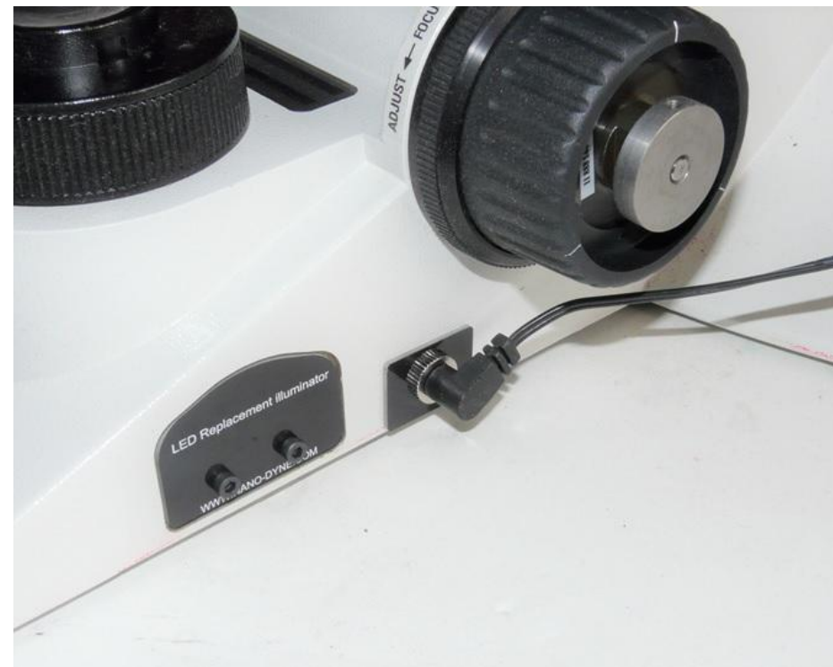
Connect the power supply to complete the illuminator installation.
