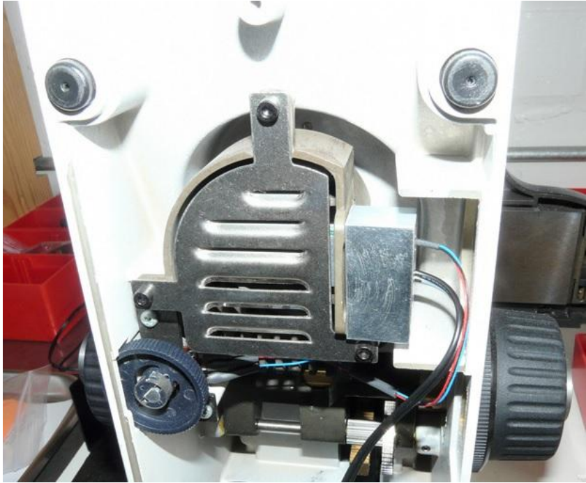
Connect a new pot cable to the Nanodyne illuminator assembly.
