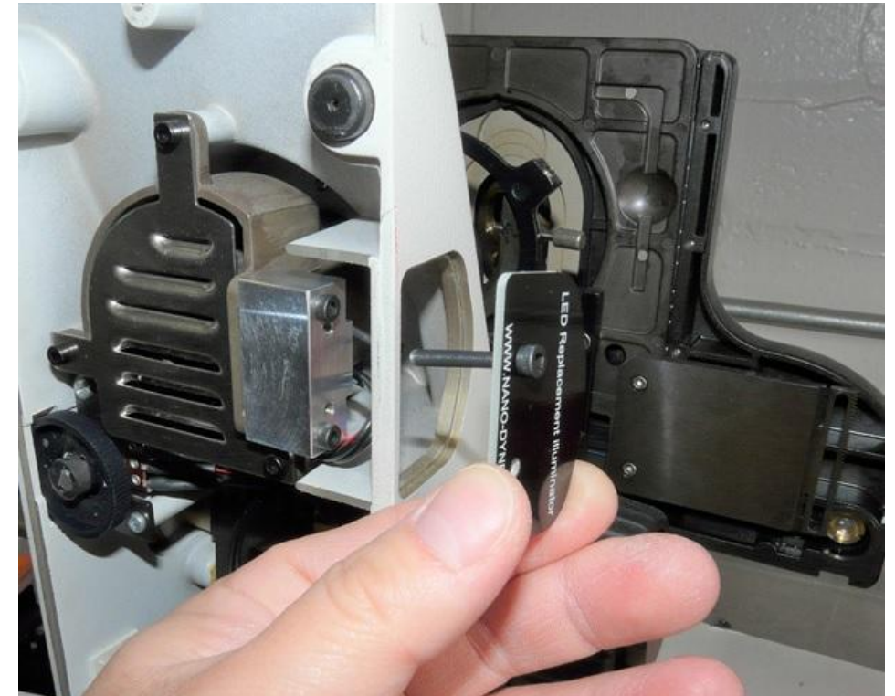
Insert Nanodyne side cover.
