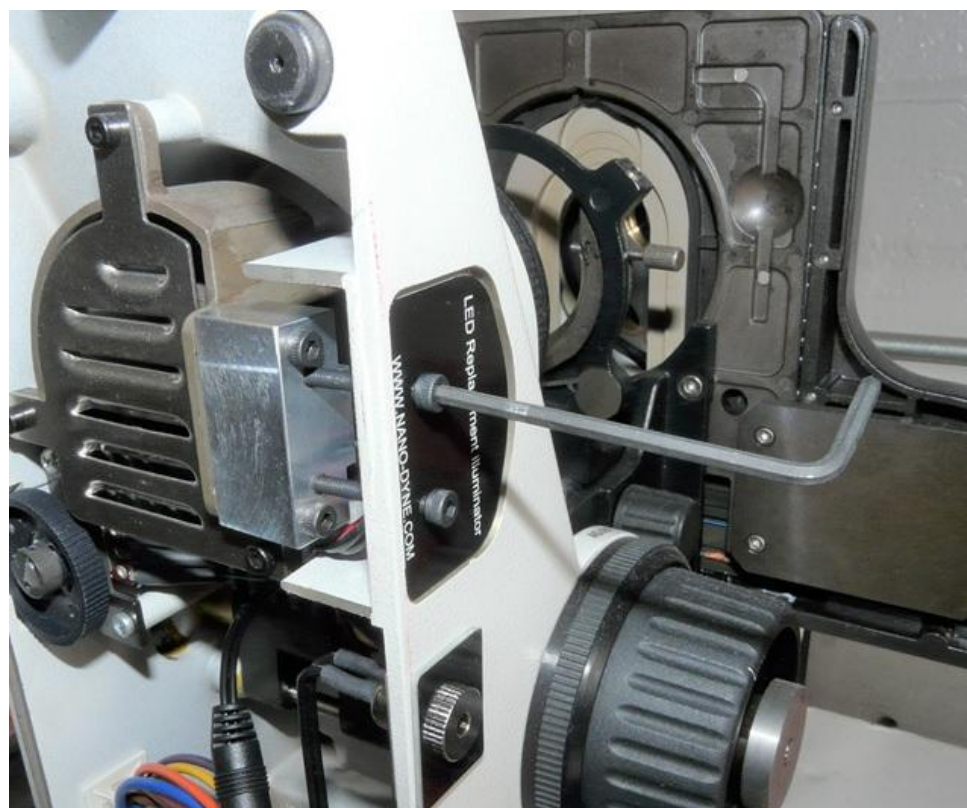
Install side cover using M3 crews provided. Do not overtighten but just enough to secure them.
