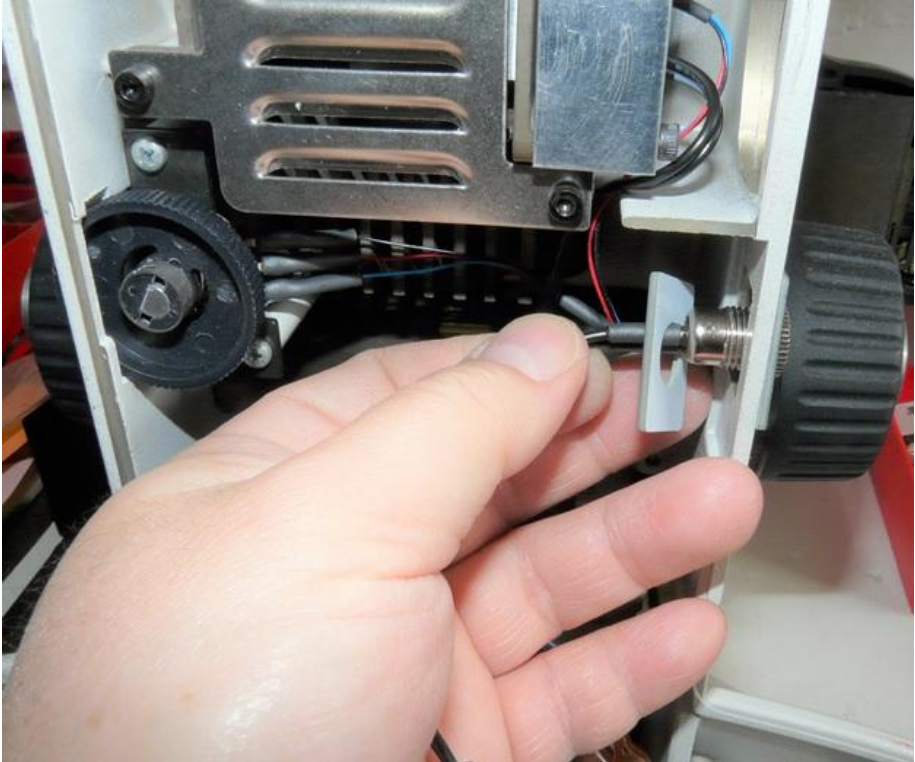
Guide the power jack and power plate outside piece through the old AC power switch hole as shown above.
