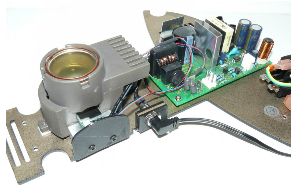
Install PN 10736 rubber plug in AC receptacle to deter connection of AC power.
