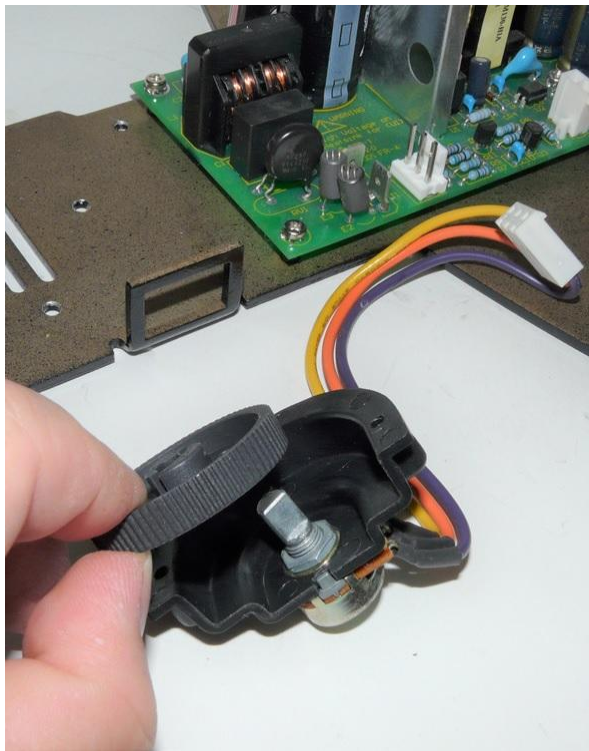
Remove the adjustment knob. Keep the knob to install on the replacement adjustment potentiometer.
