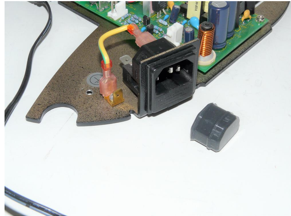
Install PN 10736 rubber plug in AC receptacle to deter connection of AC power.
