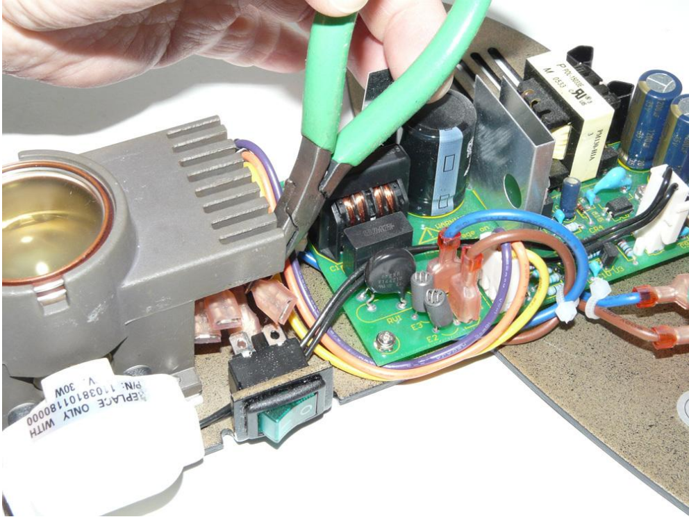
Unplug the electrical wiring from the AC switch.
