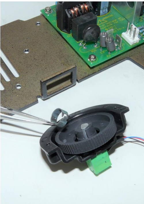
Re-install the original knob and round metal clip.
