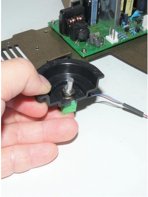
Secure the new potentiometer to the mounting bracket.
