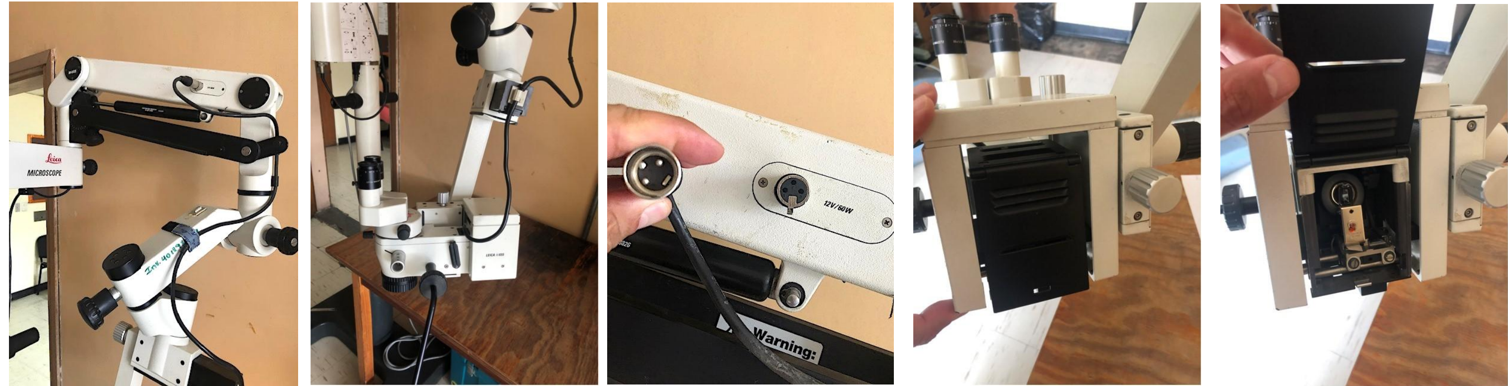
(1) Original microscope, view 1. (2) Original microscope, view 2. (3) Lamp power cable. (4) OEM lamp house from back side. (5) Back cover lifted, lamp holder visible.
