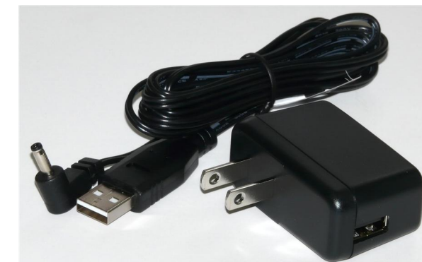
PN 10733 Power Supply - XP Power 5V 1A and PN 10734 Cable 6 foot USB A to 1.35mm ID/3.5mm OD RA Barrel Plug.
