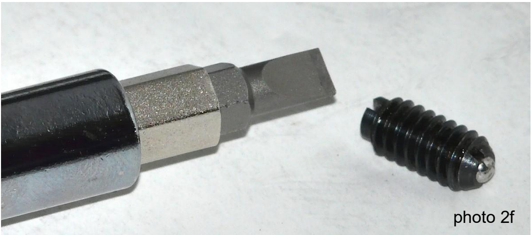
(5) Removed OEM set screw.
