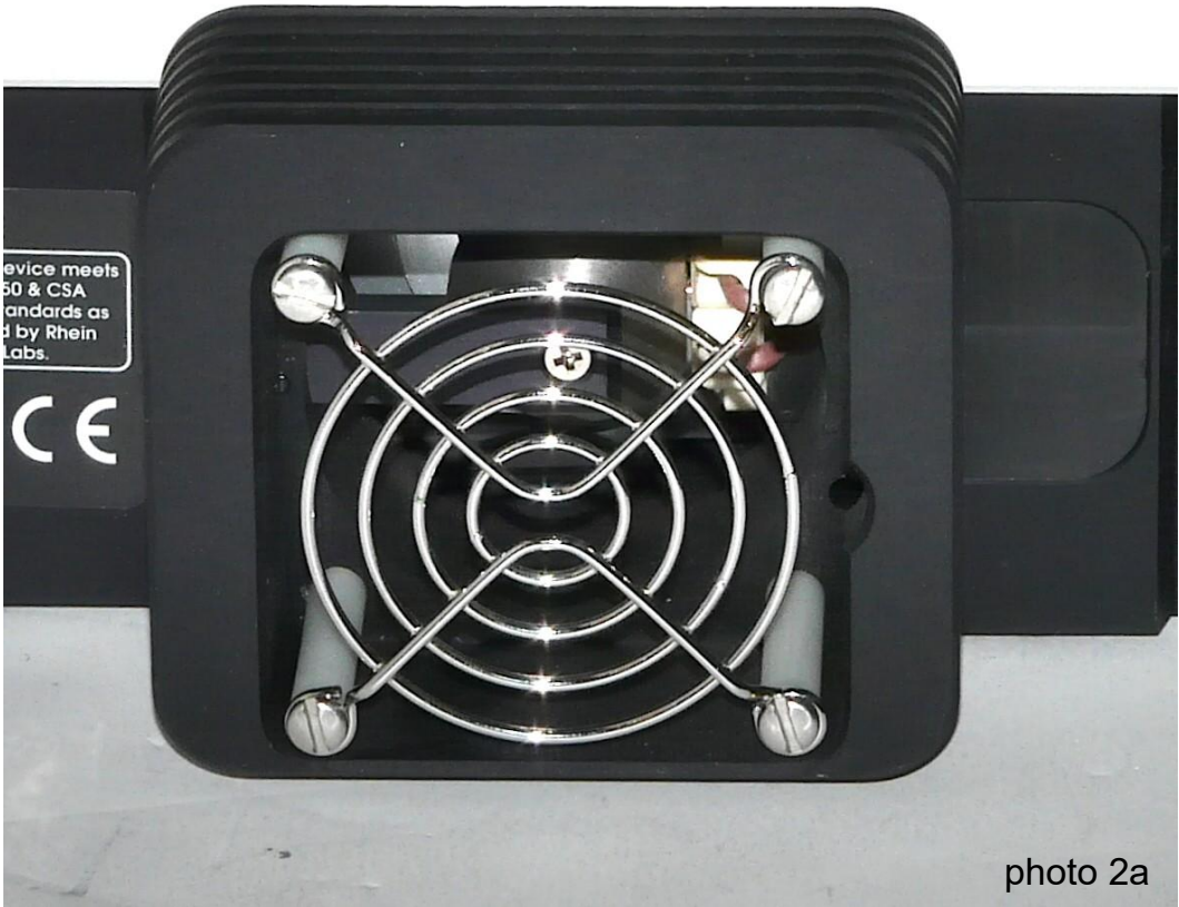
(1) Remove the metal guard from the OEM lamp housing.
