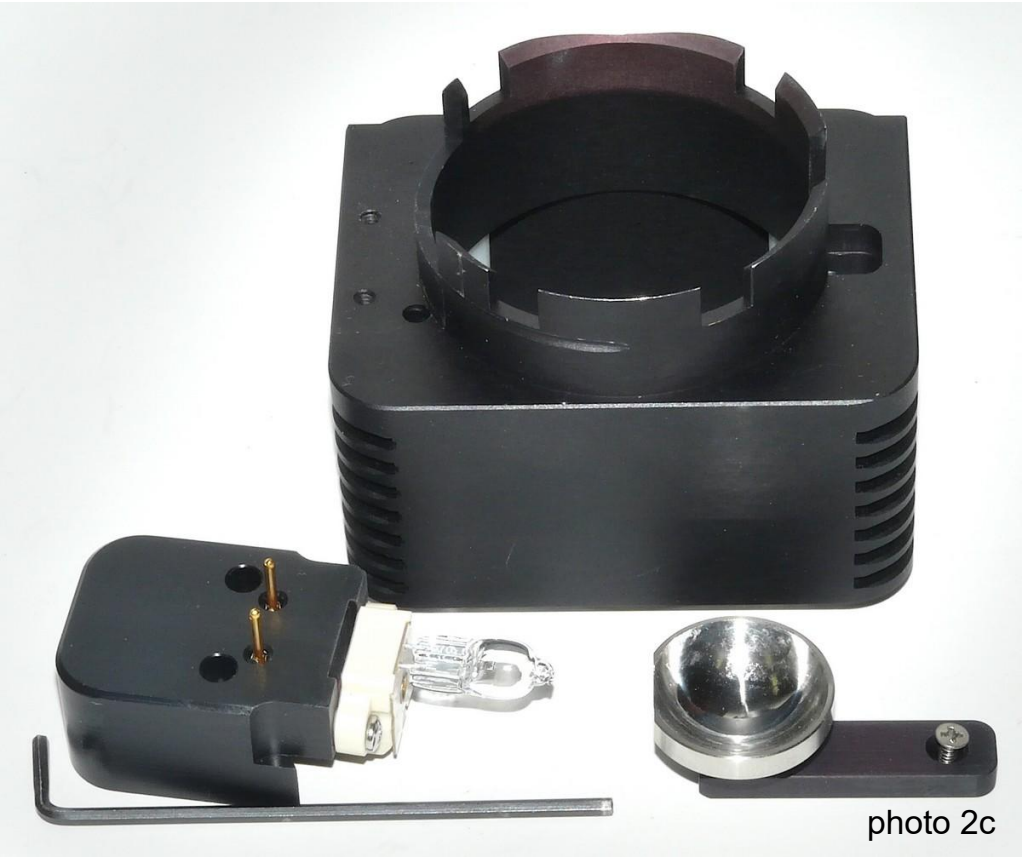
(3) Remove the OEM mirror holder as shown above.
