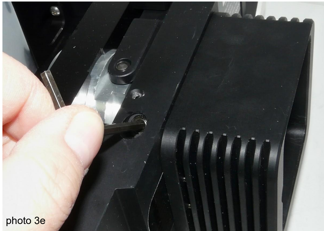
(5) Attach the OEM lamp housing as it was removed and tighten the set screw to secure Nanodyne illuminator.
