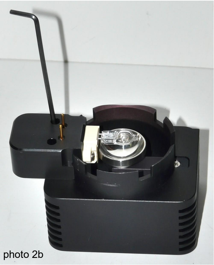
(2) Remove the lamp holder assembly. Keep the two 4-40 screws for later.
