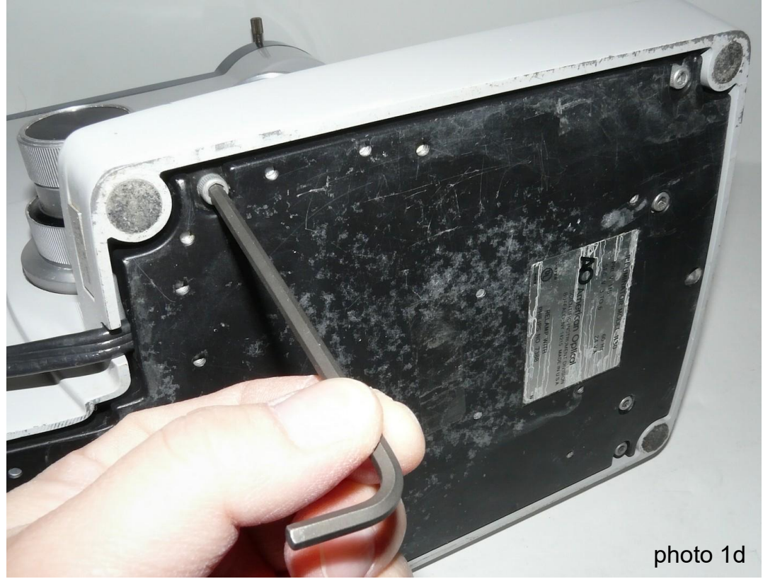
(2) Unscrew to separate the microscope base.
