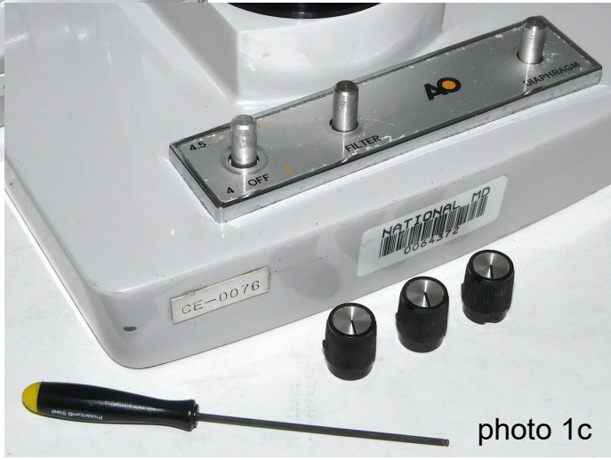
(1) Use the 0.05 inch hex key to remove the adjustment knob. Keep the knob to install on the replacement adjustment potentiometer.
