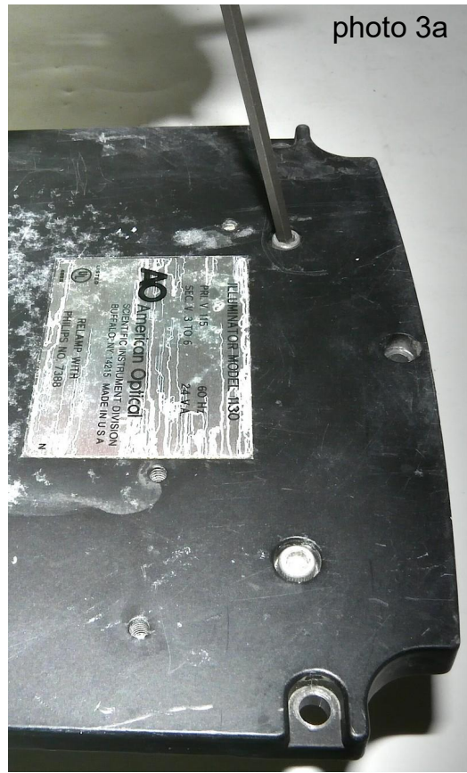
(1) Remove the two screws holding the black plastic housing to remove original potentiometer. Leave the housing in place.
