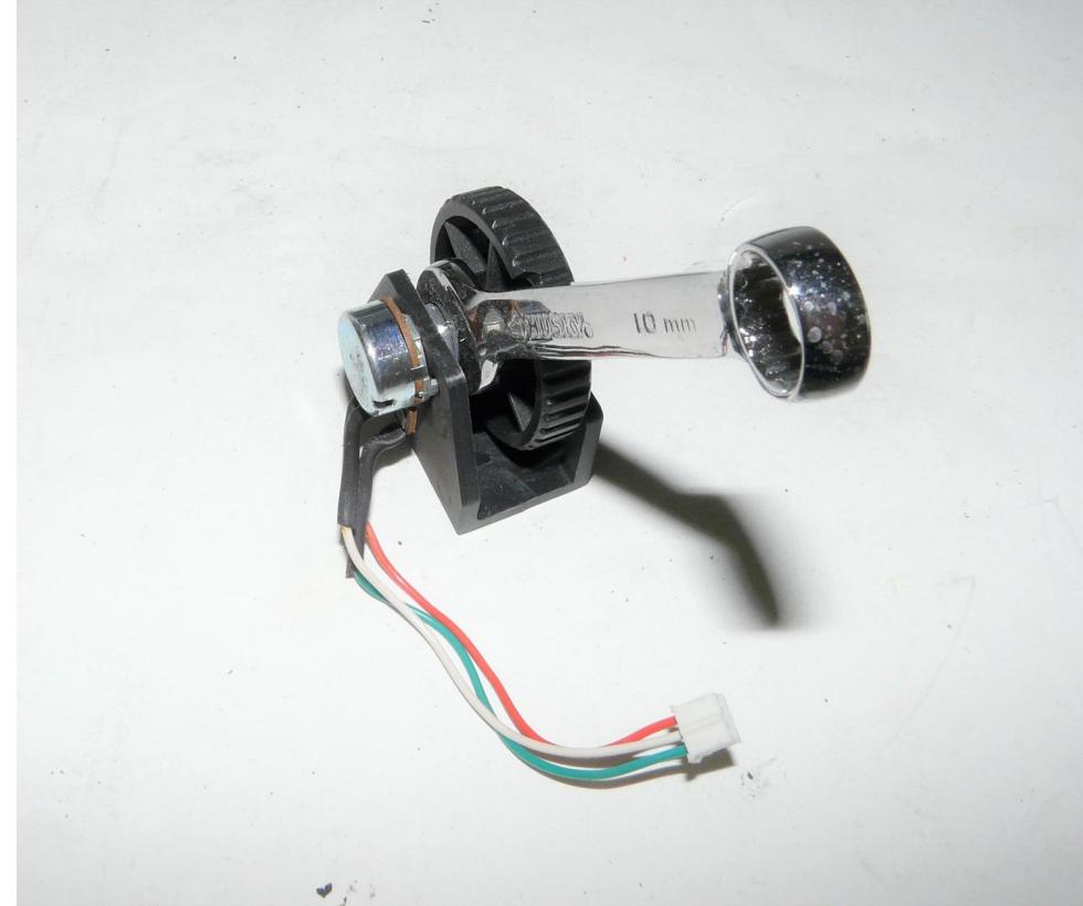
(2) Unscrew the nut holding the OEM pot, using a 10 mm hex wrench.
