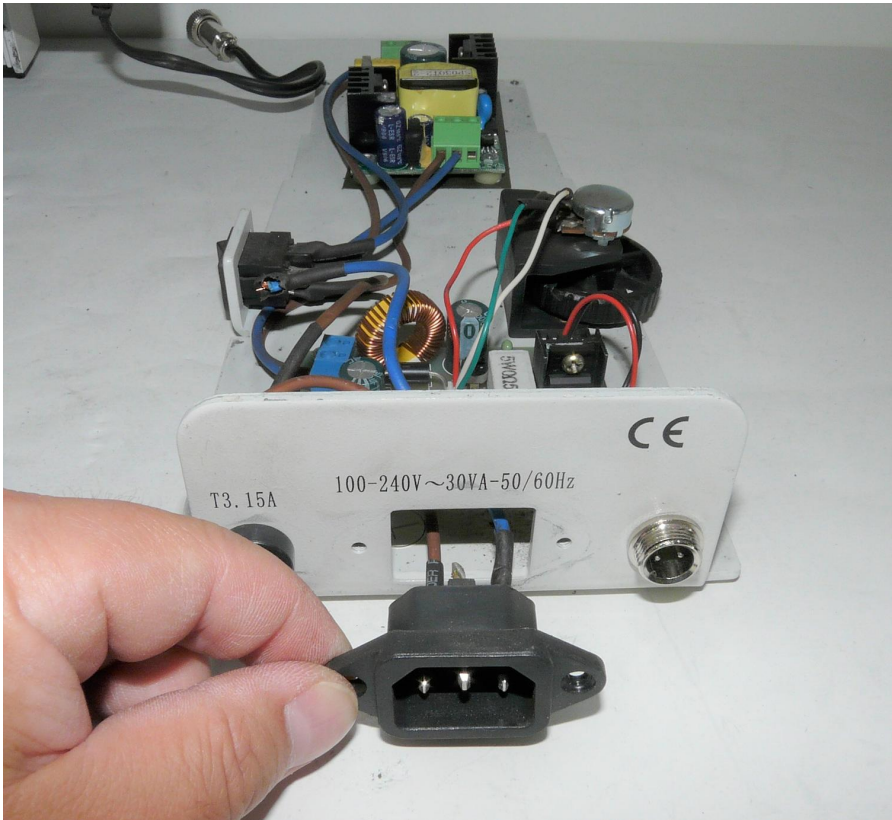
(2) Completely remove AC power receptacle out of the microscope. Nanodyne pot plate will replace it.
