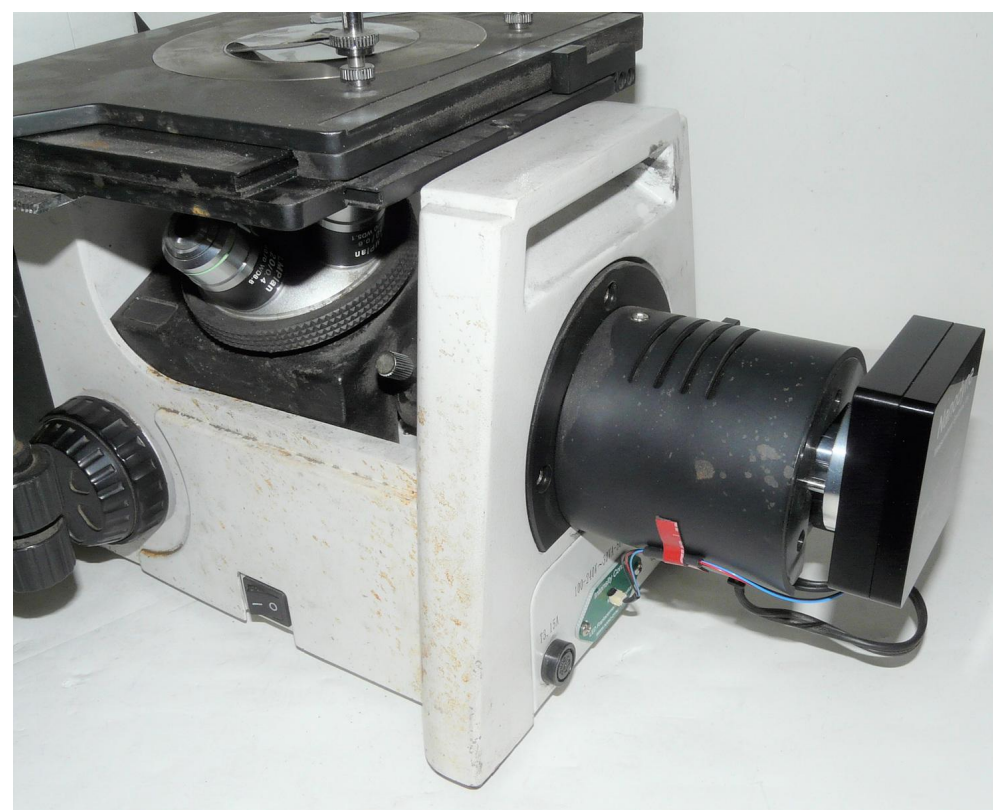
(1) Secure the pot cable with the 3M VHB tape provided (red, in above photos).
