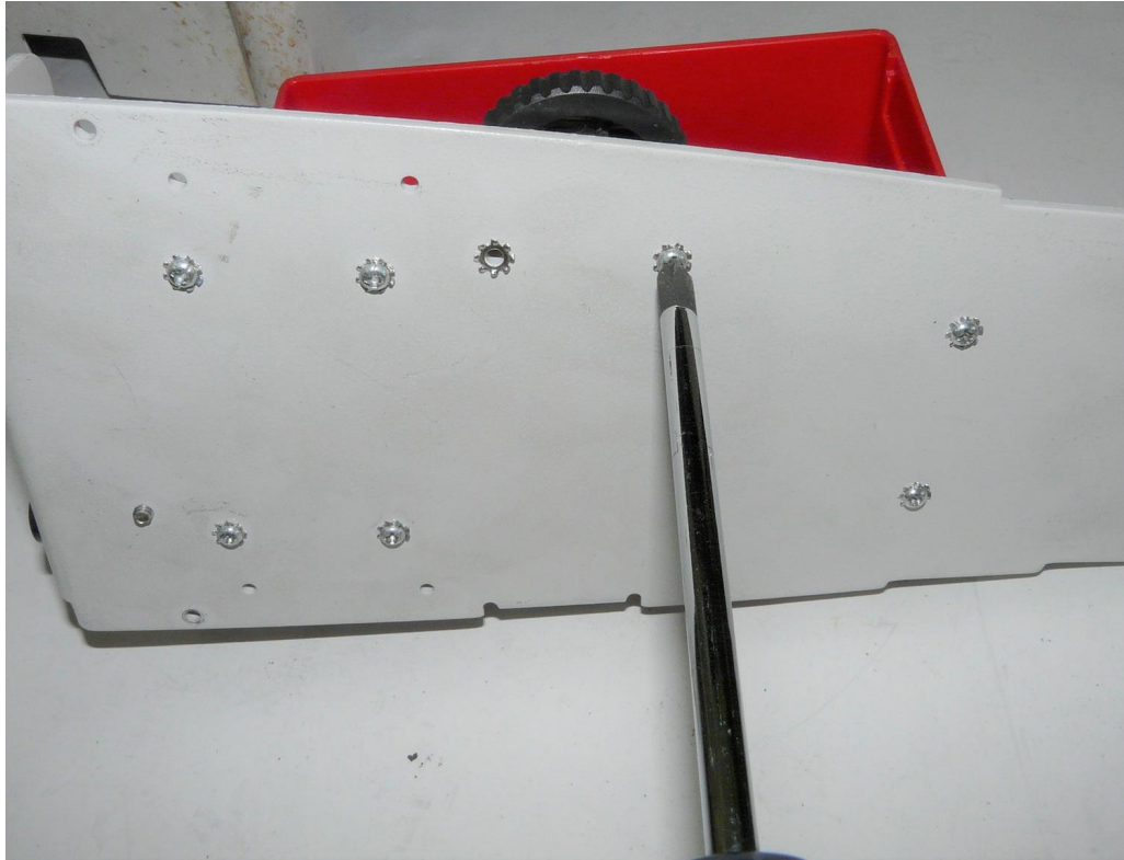
(5) Remove the bracket.
