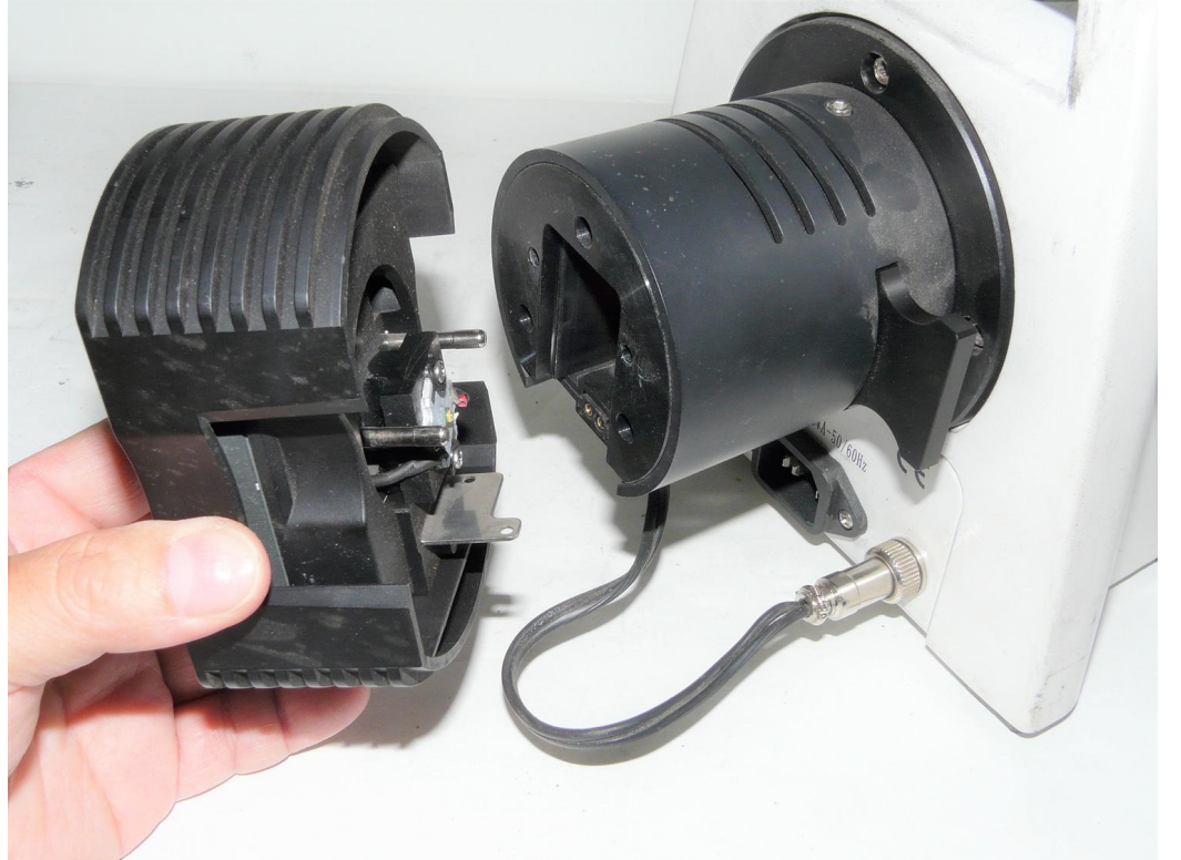
(3) Remove the original lamp.
