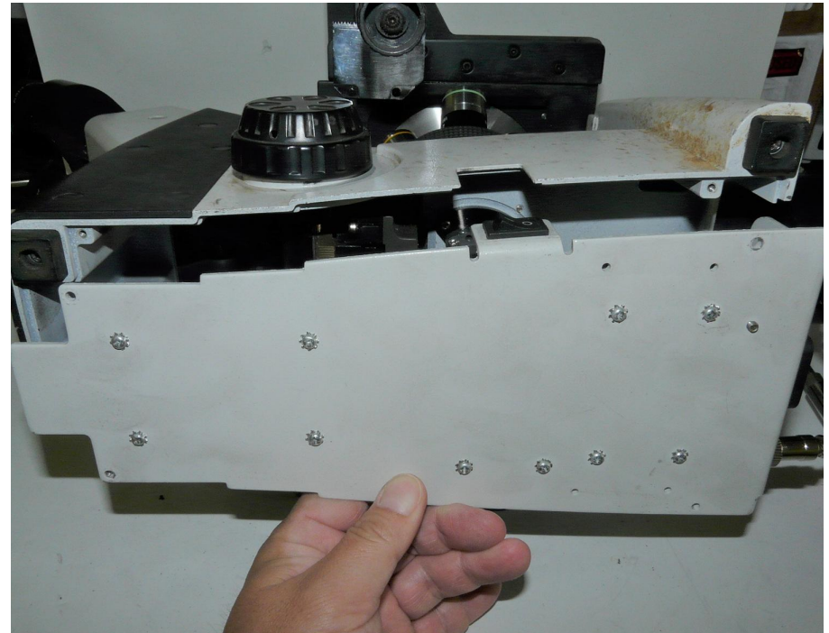
(4) Remove the 4 screws holding bottom cover using screw driver and open the bottom cover. Keep the screws for later.
