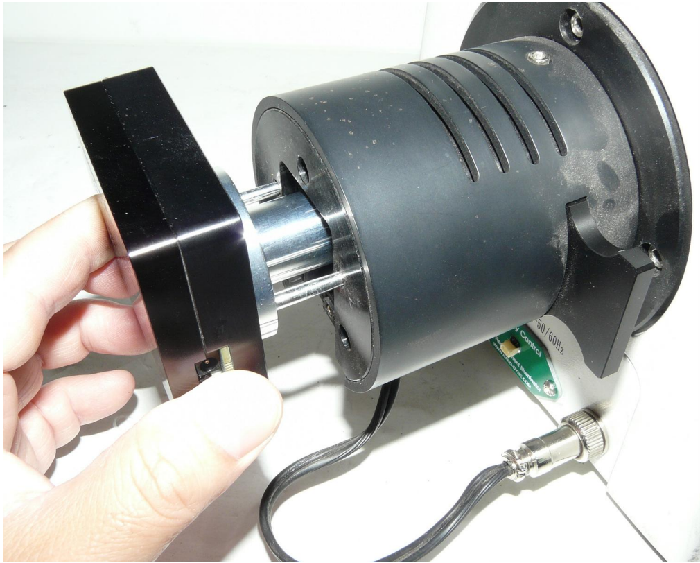
(1) Insert the new illuminator.
