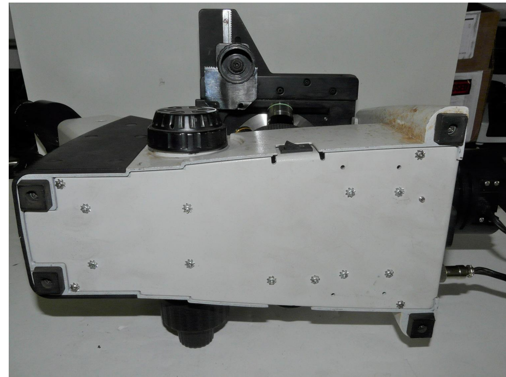
(4) Remove the 4 screws holding bottom cover using screw driver and open the bottom cover. Keep the screws for later.
