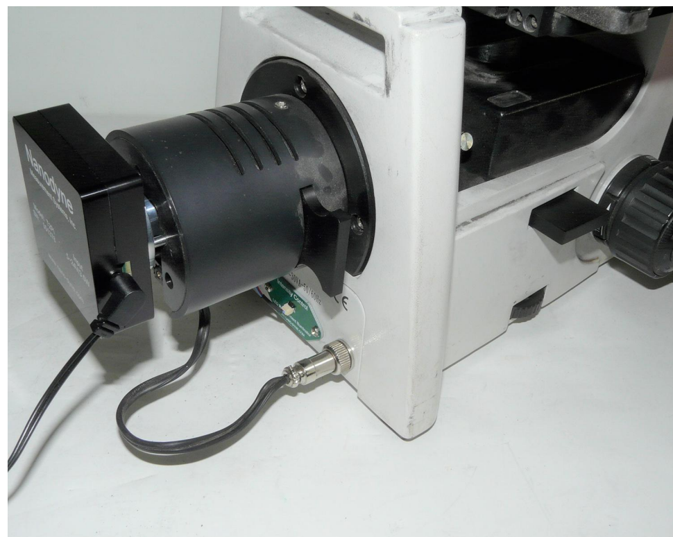
(3) Connect the USB end of the power cable to the power supply. Plug in the other end of the power cable to the illuminator.
